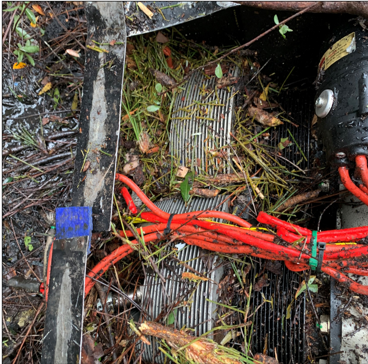
Photo 3: View of chopped pine tree fragments located at the top and rear section of engine
