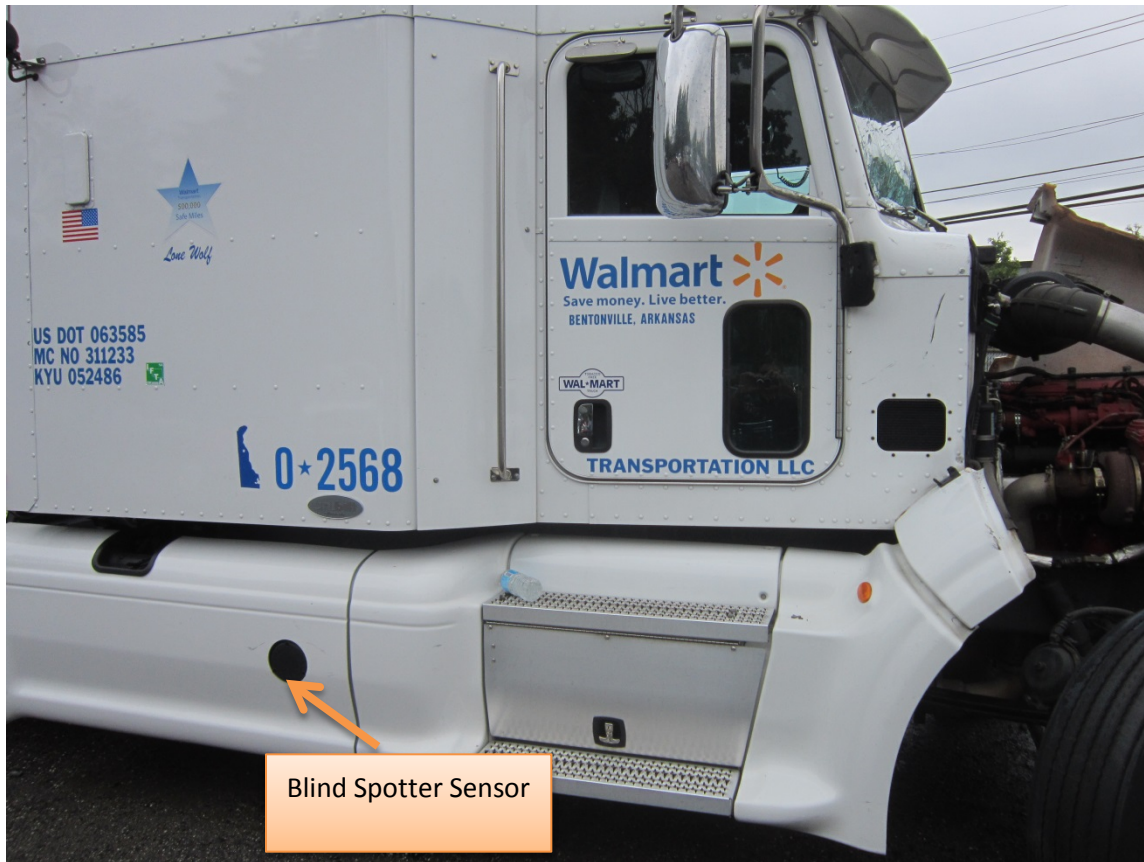
Photo 8: This photo depicts the Blind Spotter that was located on the right side (passenger side) of the Walmart accident truck-tractor.
