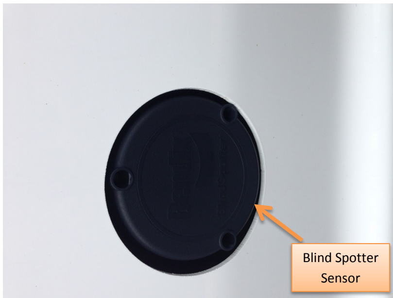
Photo 9: This photo depicts a close up view of the Blind Spotter Sensor located on the Walmart accident truck tractor
