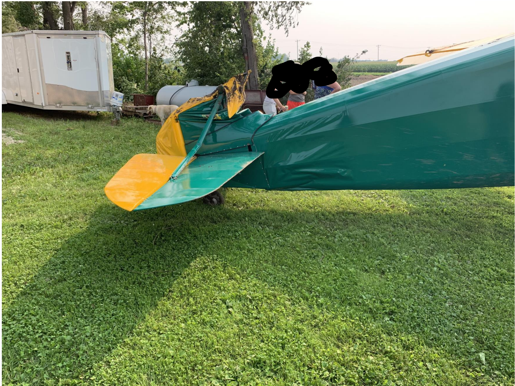
Photo 2 – Damaged tail section
