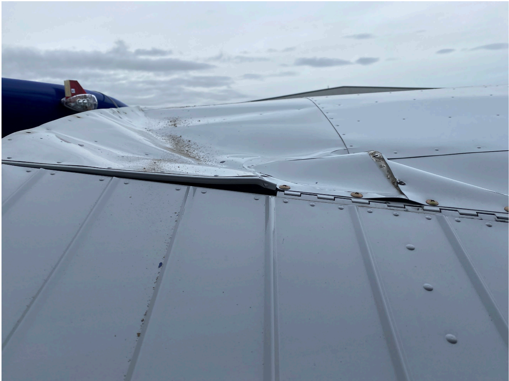
Photo 1 – View of the left wing damage. Courtesy of the FAA.
