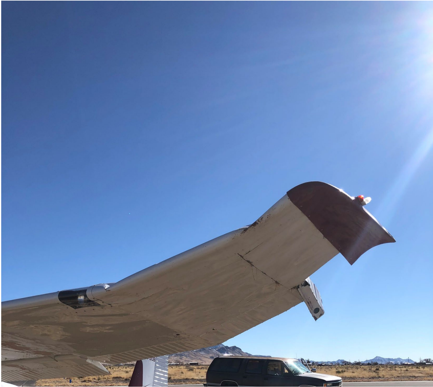
Photo 2 - N4750B Left Wing Damage, Courtesy owner
