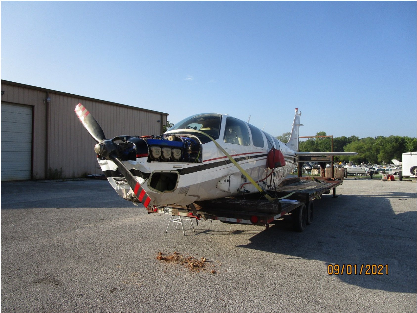
Photo 2 – Accident airplane prepared for an engine test run
