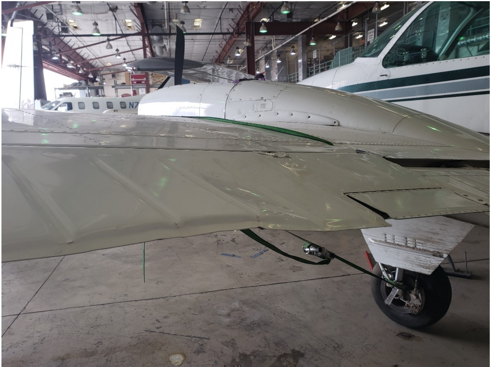
Photo 1 – View of the left aileron damage. Courtesy of the FAA.
