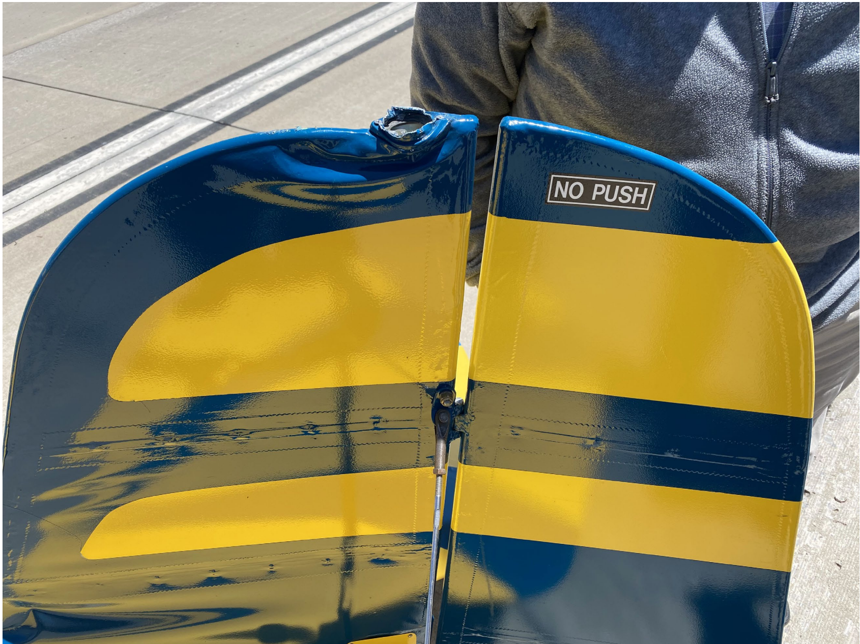
Photo 2 – Damage to vertical stabilizer
