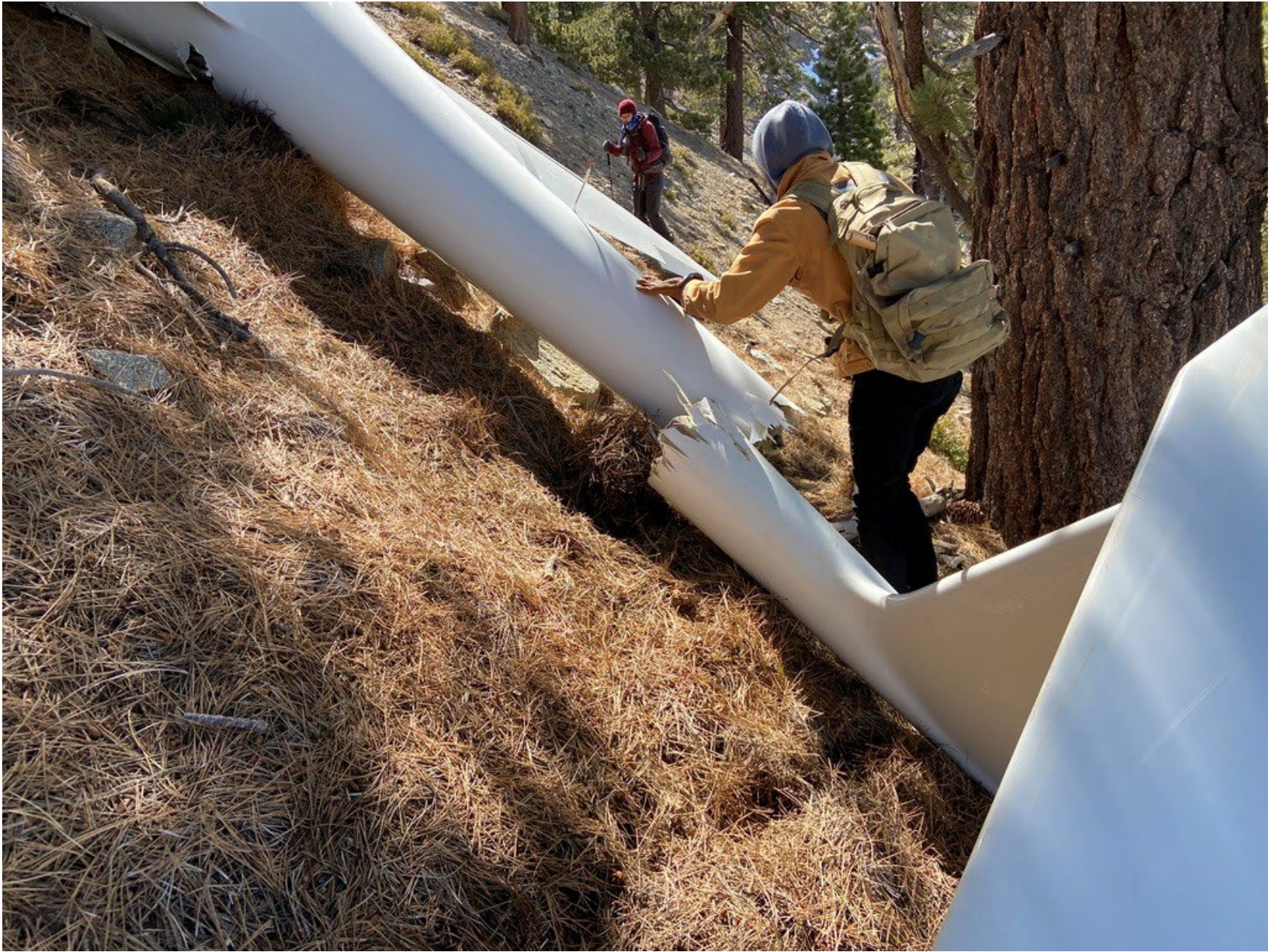
Photo 6 – Damaged Tail (Photo Courtesy of Operator)
