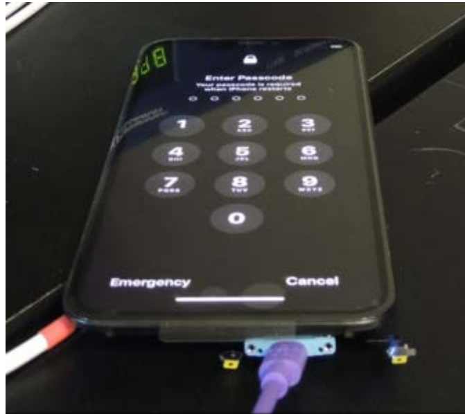
Figure 8: Motherboard of Apple iPhone XR powered up in a surrogate device.
