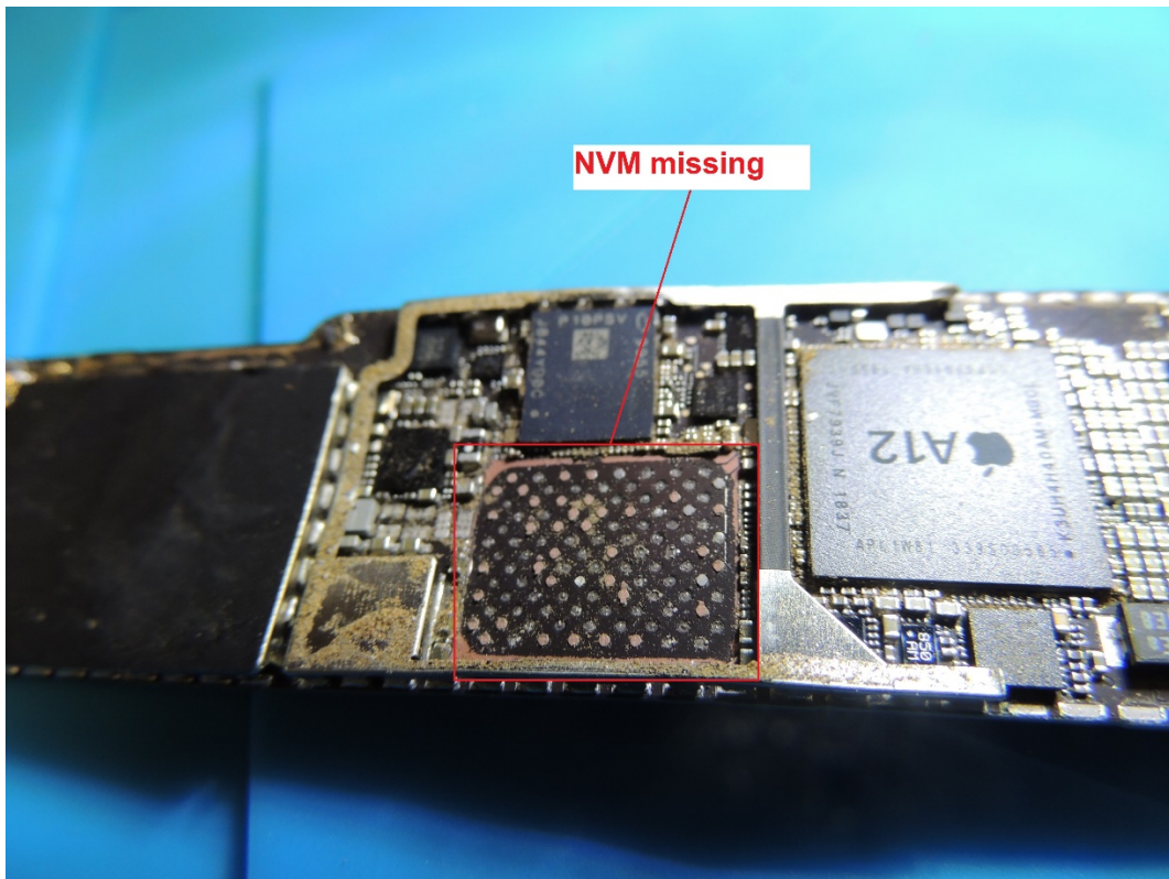
Figure 2: Location of the missing NVM on the motherboard of Apple iPad Mini 5.
