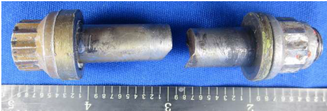
The fractured bolt found on Bell 407 S/N 53563. (Image courtesy of Bell)
