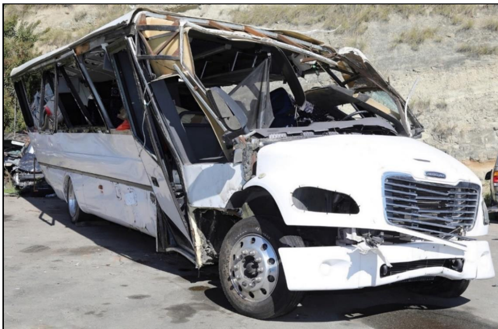
Figure 8. View of damage to front and right side of bus.
