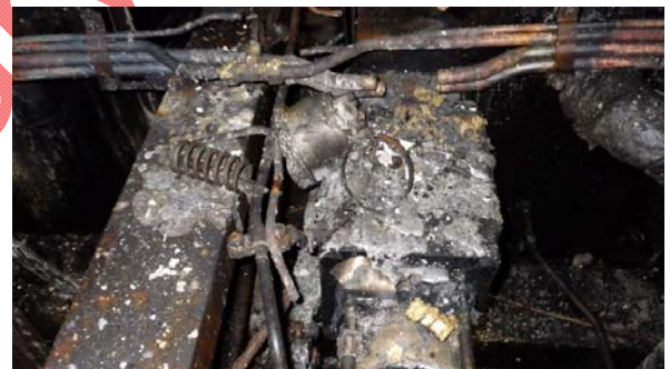
VIT Cylinder melted, remaining laying on top of housing for reversing mechanism.
