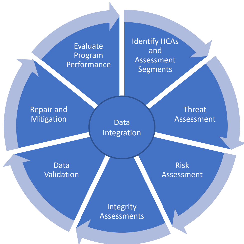
Figure 10. Integrity management process flow.
