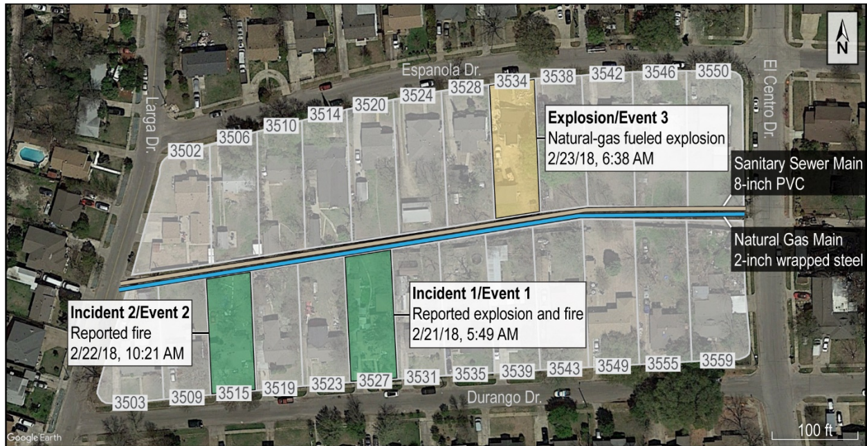
Figure 1. Location of explosion, preceding incidents, and shared utilities.
