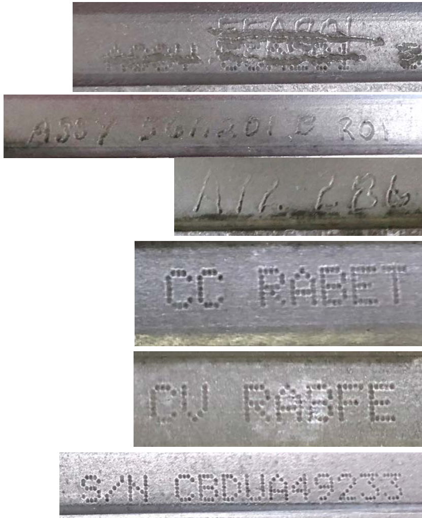
Figure 96: Image showing the following sister blade, CBDUA49233, the part markings, and the pieces recovered from the ground that were found to be remnants of this blade.
