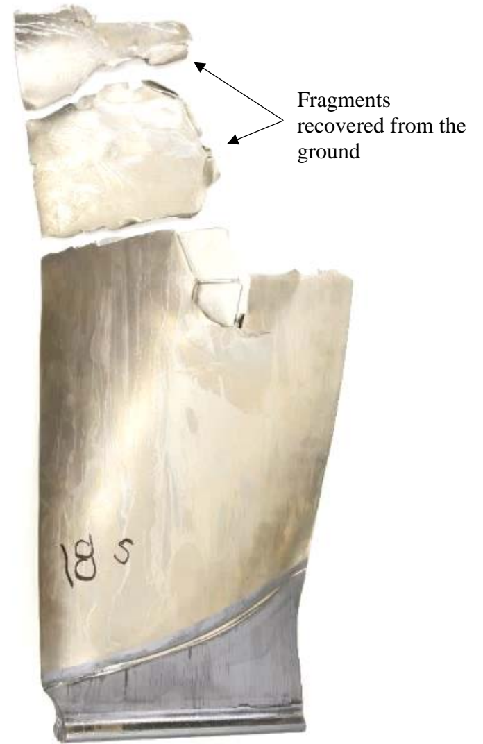
Figure 96: Image showing the following sister blade, CBDUA49233, the part markings, and the pieces recovered from the ground that were found to be remnants of this blade.
