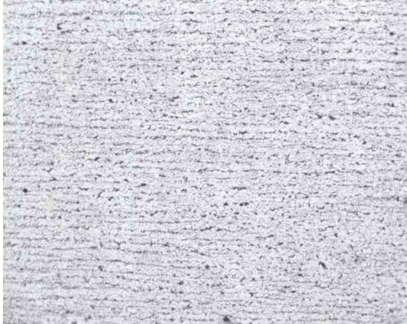
Photograph 7. Representative microstructural features of the pipe steel at MP 487.5 with fine-grained, banded ferrite and pearlite. 100X. Nital reagent.
