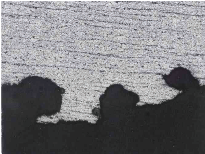
Photograph 12. Representative microstructural features of the pipe steel at MP 496.9 OD surface corrosion in the form overlapping pits. 100X. Nital reagent.
