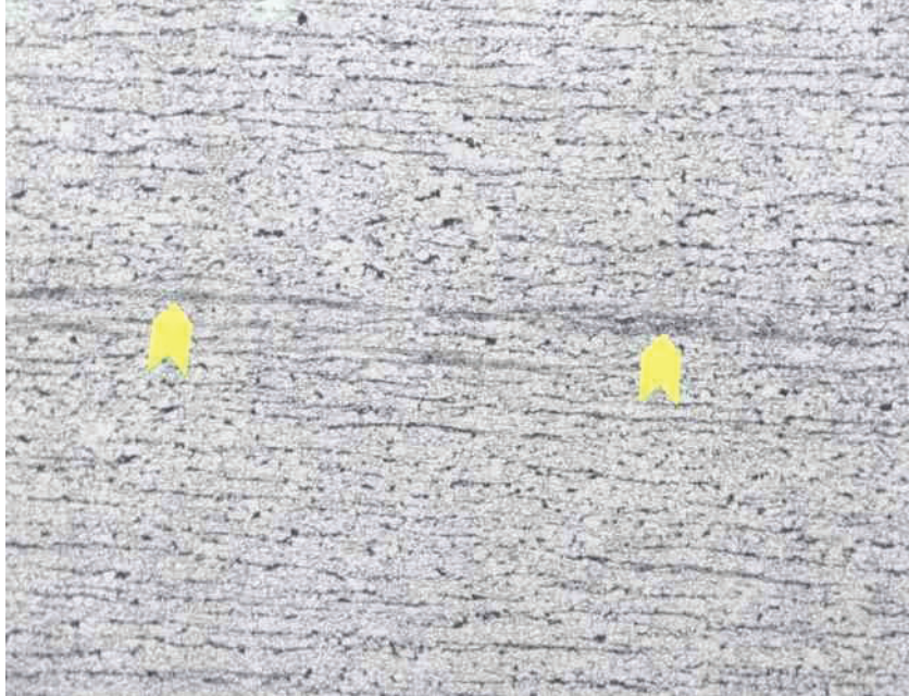
Photograph 11. Representative microstructural features of the pipe steel along the rupture interface at MP 487.5 showing some minor inclusion clusters (arrows). 100X. Nital reagent.
