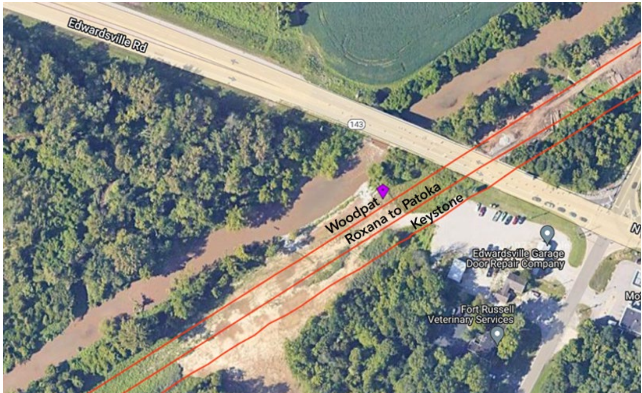
Figure 3. The Woodpat 22-inch pipeline, Roxana to Patoka 12-inch pipeline, and Keystone 30-inch pipeline, are shown north to south, in a shared ROW adjacent to the Cahokia Creek, the purple diamond shows the failure location. (Source: National Pipeline Mapping System.)
