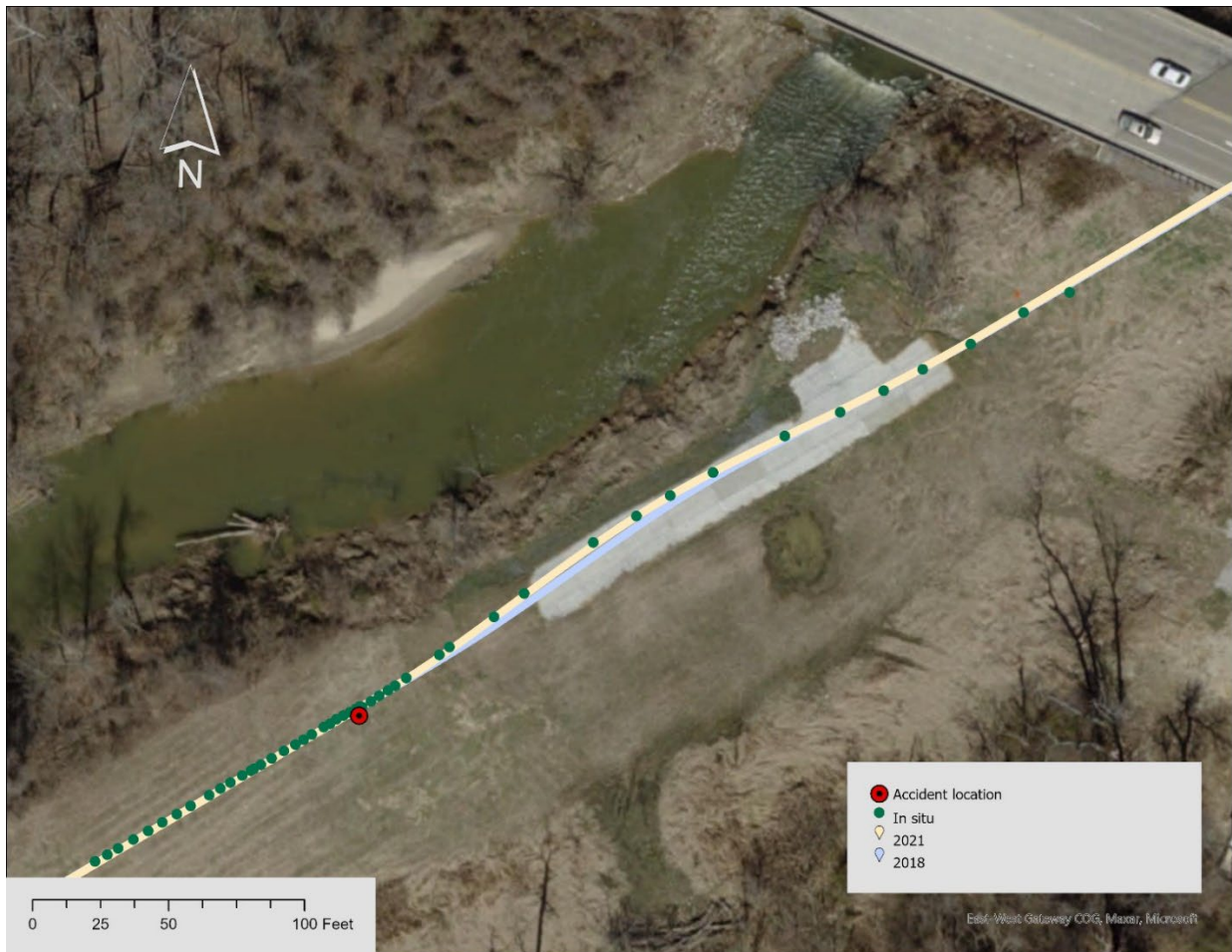
Figure 4. GPS survey locations compared to 2018 and 2021 IMU data with a red dot indicating the accident location.
