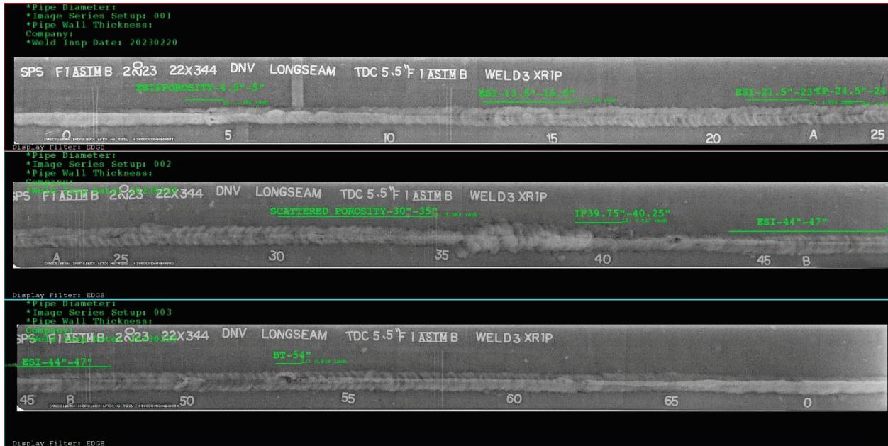
Figure 3: RT image of intact girth weld.
