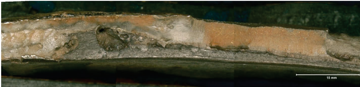
Figure 2: Photograph of fracture surface.
