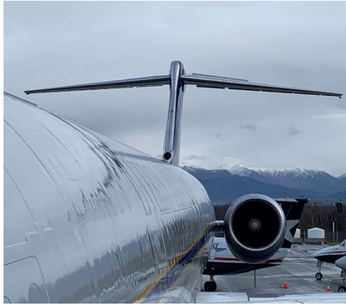
Figure 1. Elevator as viewed from airstairs at the main cabin entry door located on the left (captain's) side of the airplane.
