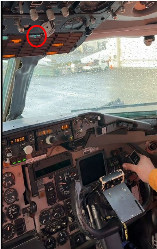
Figure 9. Elevator Power On blue overhead light (circled in red above) activation with control column in full forward position.
