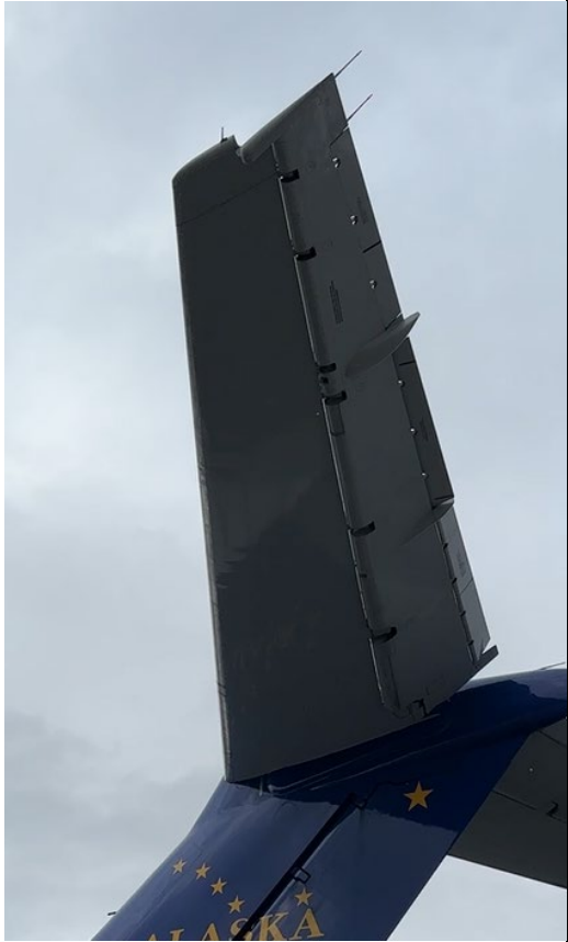
Figure 13. Left side (captain's side) elevator as viewed from the ground in the trailing edge up position.
