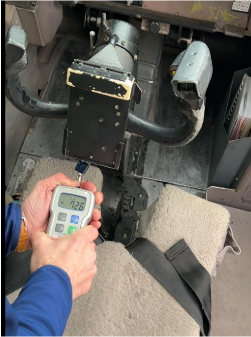
Figure 15: Full aft pressure applied during a normal non-jammed elevator flight control check.
