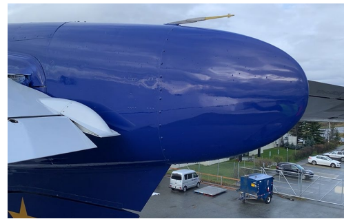
Figure 8. Elevator as viewed from the left side (captain side of airplane) with control column aft pressure being applied in the cockpit. In the photo manual downward pressure is being applied to the left side of the elevator to remain in trailing edge down.
