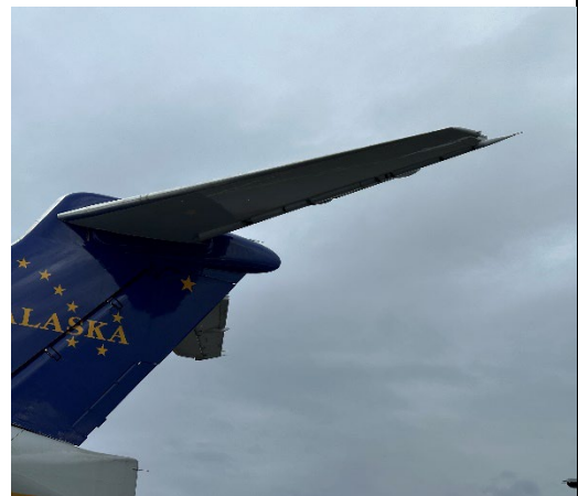
Figure 12. Left side (captain's side of airplane) elevator with full aft control column pressure.
