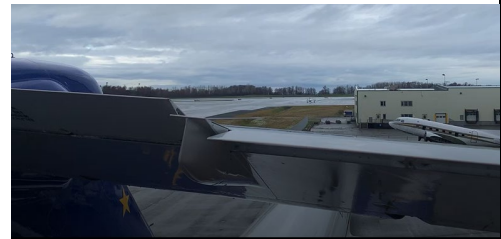
Figure 4. Elevator as viewed from an elevated position, in trailing edge up position.
