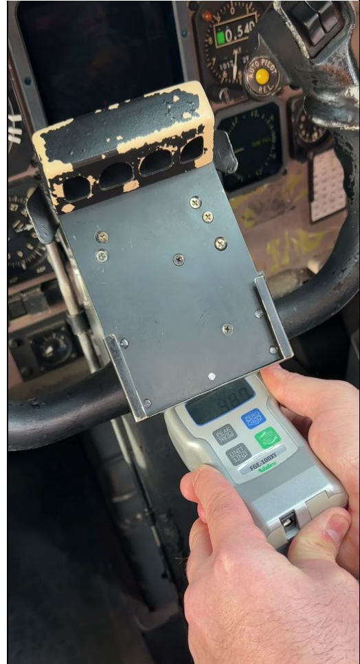
Figure 16: Full forward pressure applied during a normal non-jammed elevator flight control check.
