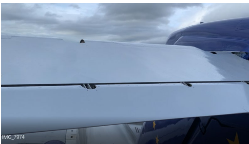
Figure 11. Left side (captain's side) elevator in trailing edge down with full forward control column.
