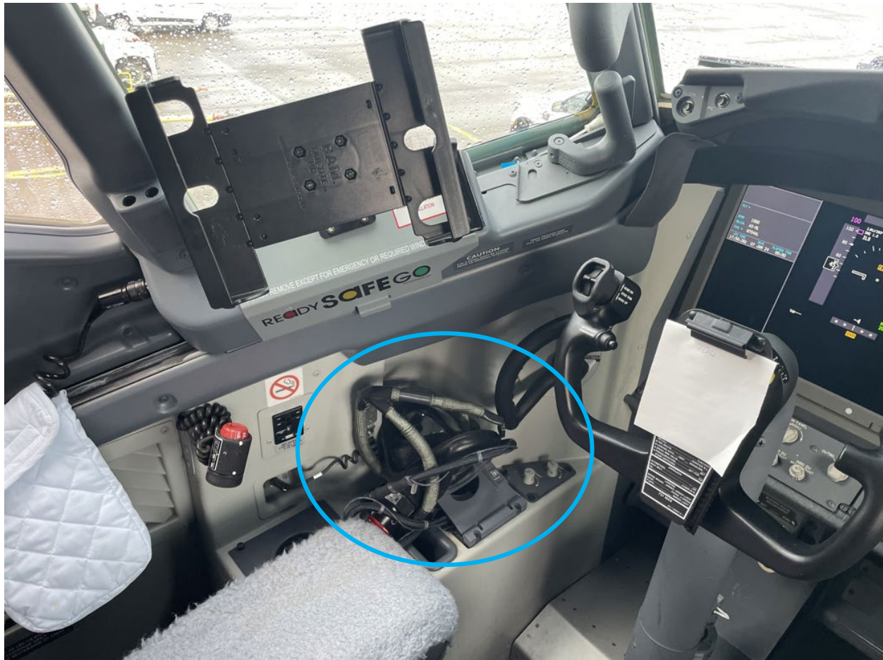
Figure 7. Captain side panel of accident airplane with oxygen mask and stowage box indicated by blue circle. (Source: NTSB)
