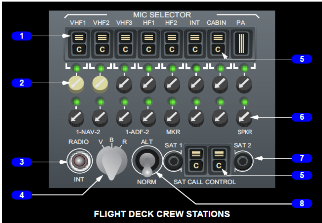
Figure 11. 737-9 Audio Control Panel (Source: Alaska SH)
