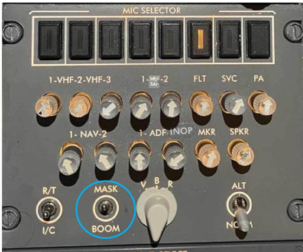
Figure 12. 737 NG ACP. Mask/Boom switch indicated by blue circle (Source: NTSB)
