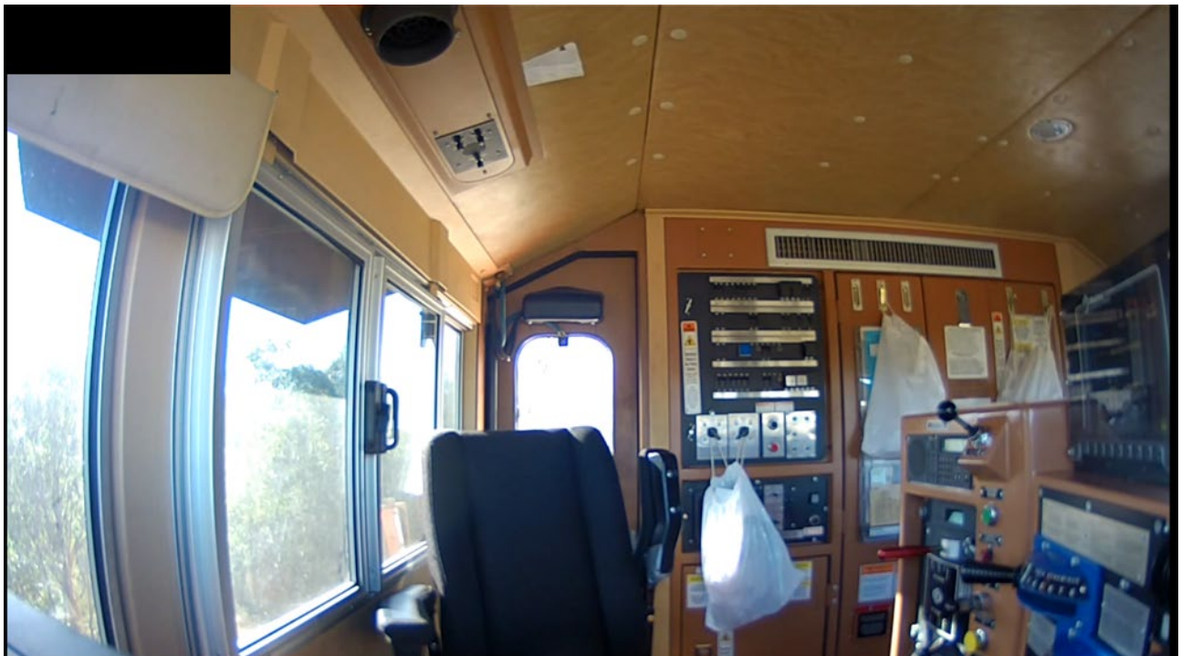
Figure 1: Camera view of the control stand and engineer seat of the lead locomotive.
