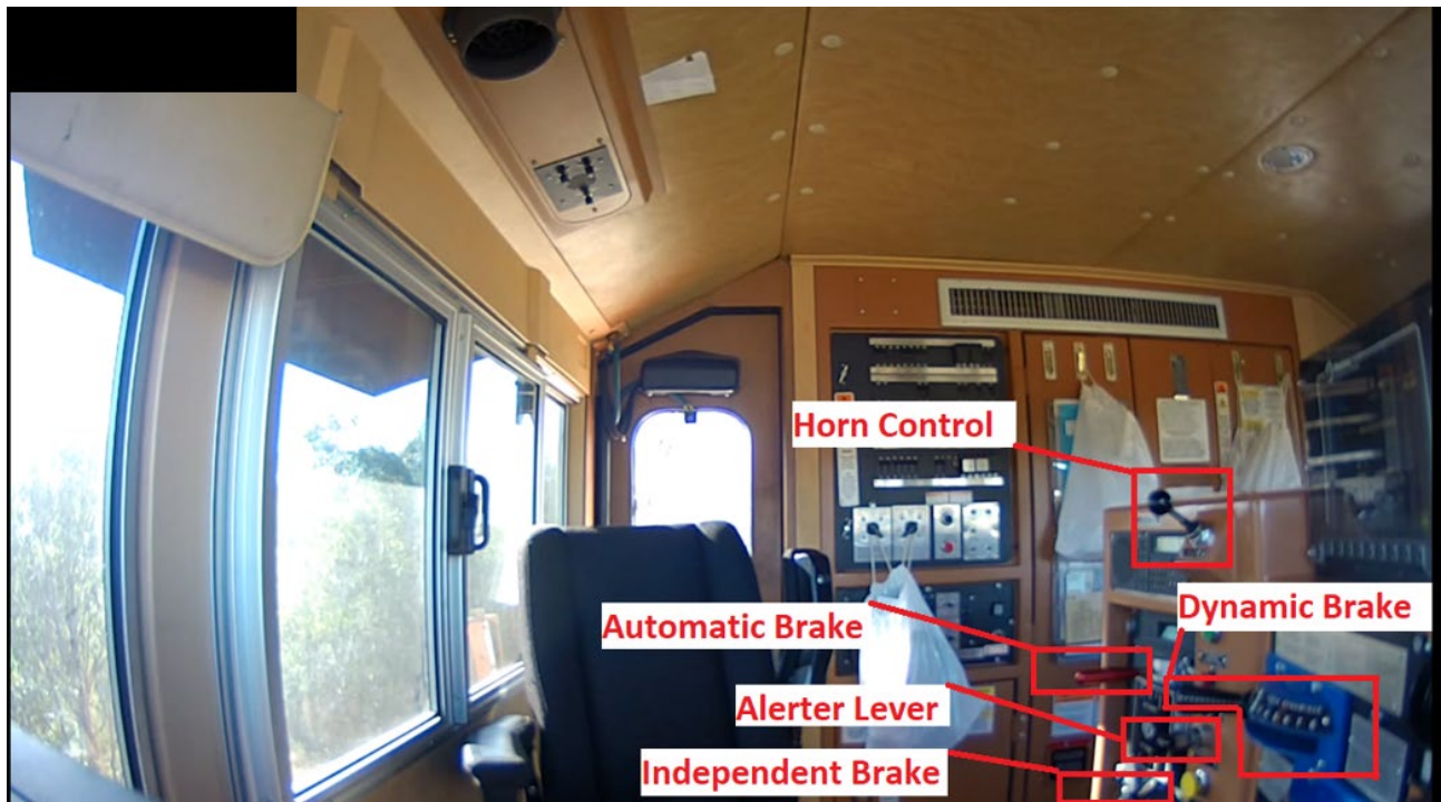
Figure 2: Camera view of the control stand and engineer seat of lead locomotive with annotations on the control stand.
