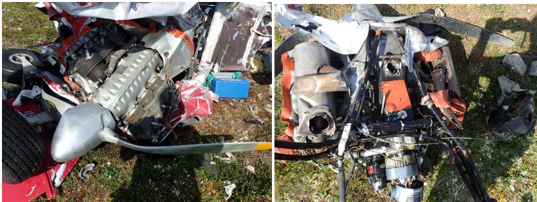
Figure 3. Continental O-300 engine and attached propeller upright (left) and bottom (right) at the accident scene.
