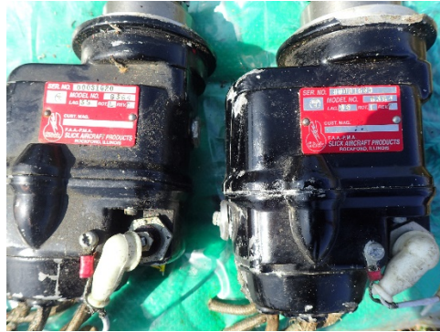
Figure 4. Left and right magnetos removed from the engine accessory drive.
