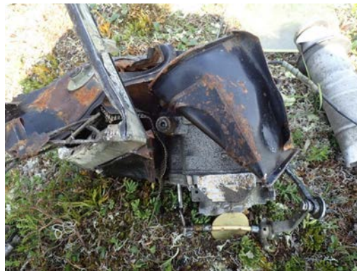
Figure 6. Carburetor and airbox at the accident scene.
