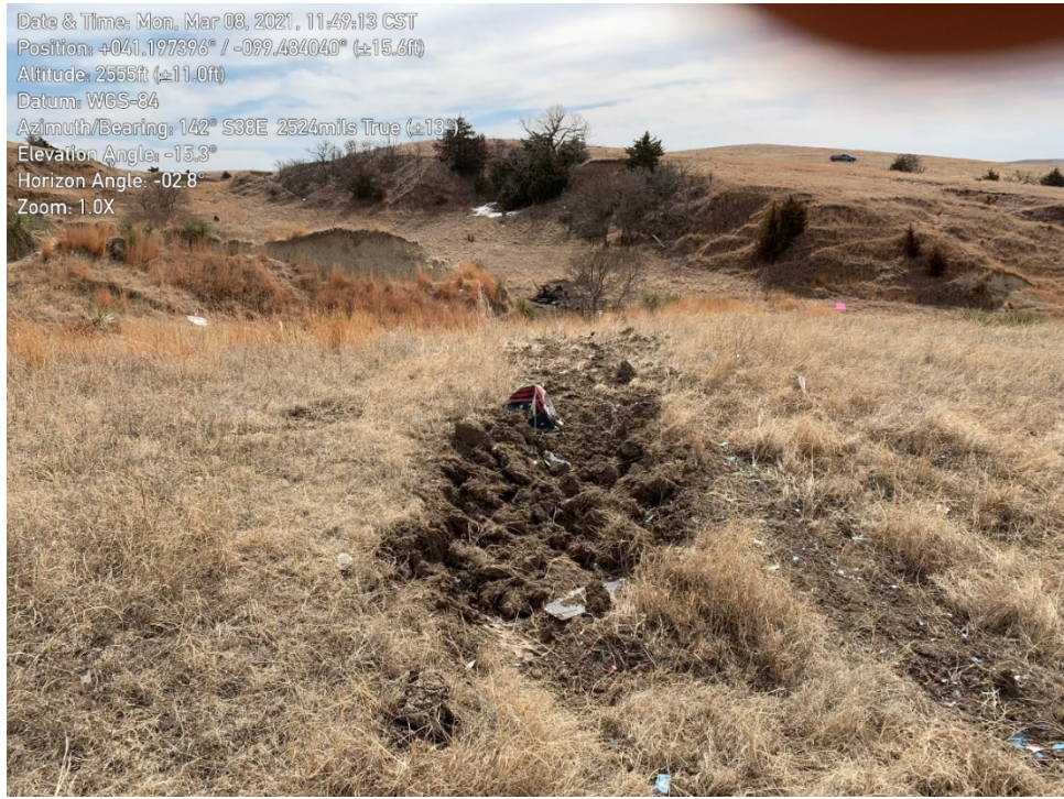
Figure 4: Large Area of Disturbed Dirt with Propeller Blade Fragments
