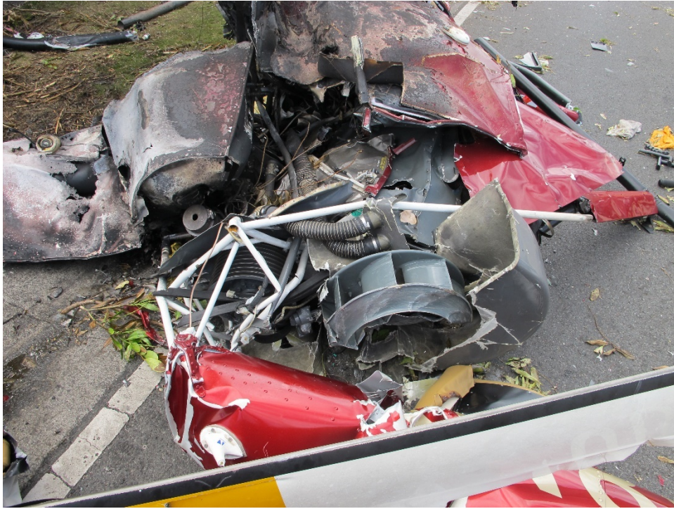
Figure 7: Upper Sheave and Cooling Fan
