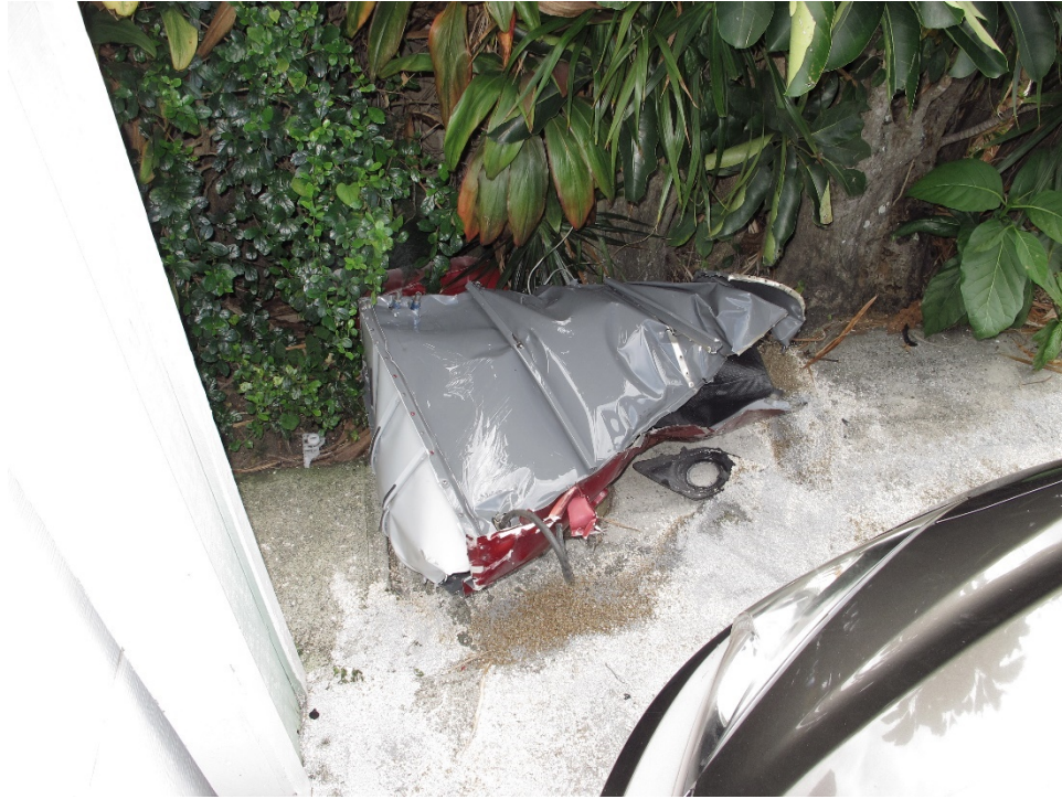
Figure 9: Main Fuel Tank
