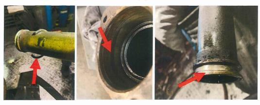
Below are both pieces of the 109-2332 seal-o-ring. The smaller piece was found on top of the front cover. The front cover is directly below the upper joint area where the tube is attached to the oil filter housing. The seal-o-ring doesn't show any flat area's that would indicate that this seal has a high amount of running hours on it.
