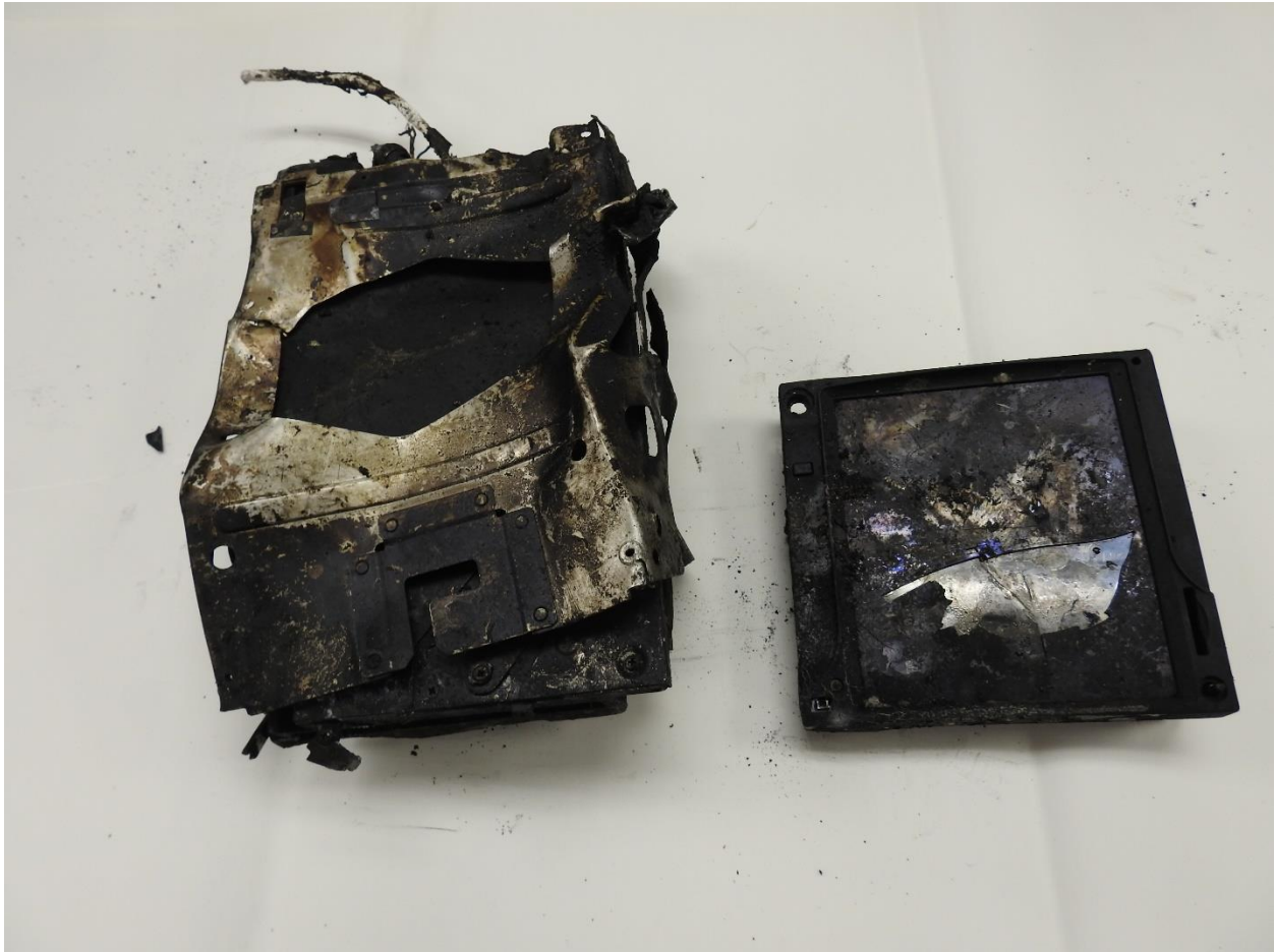
Figure 1. The Garmin GTN 750 as received, the main body on the left and the screen on the right.
