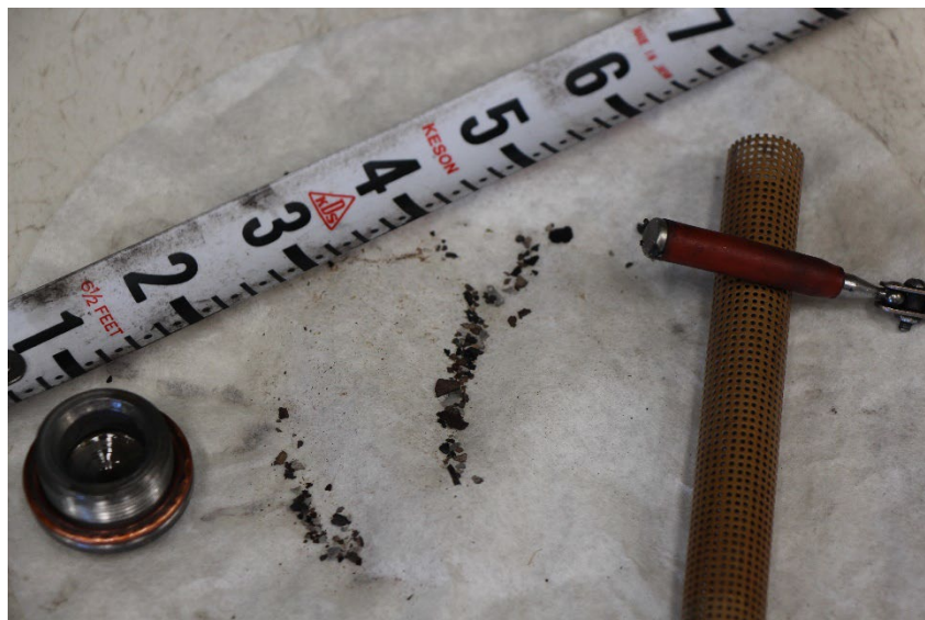
Photograph 9: Oil suction screen particles removed from screen
