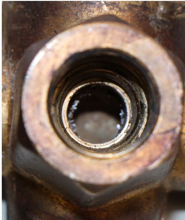
Photograph 4: Engine port with particles
