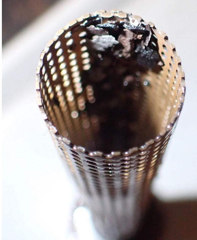
Photograph 8: Oil suction screen and particles
