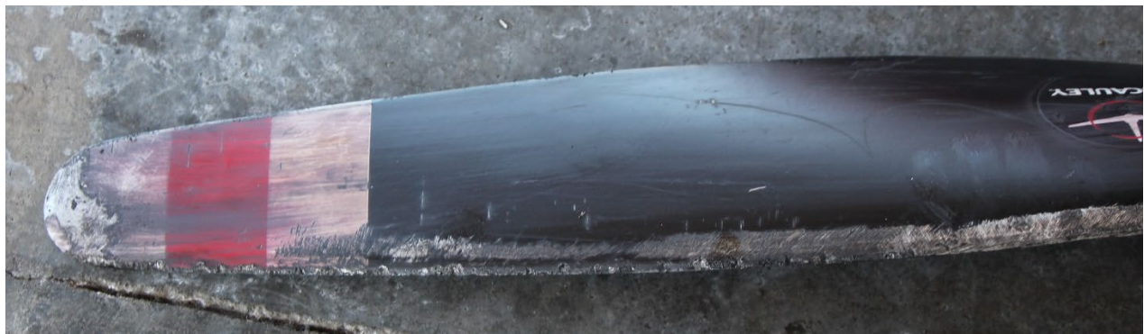
Photograph 11: Blade B nicks and gouges and leading edge
