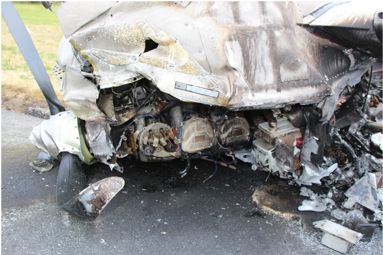
Photograph 6: Engine compartment at accident site
