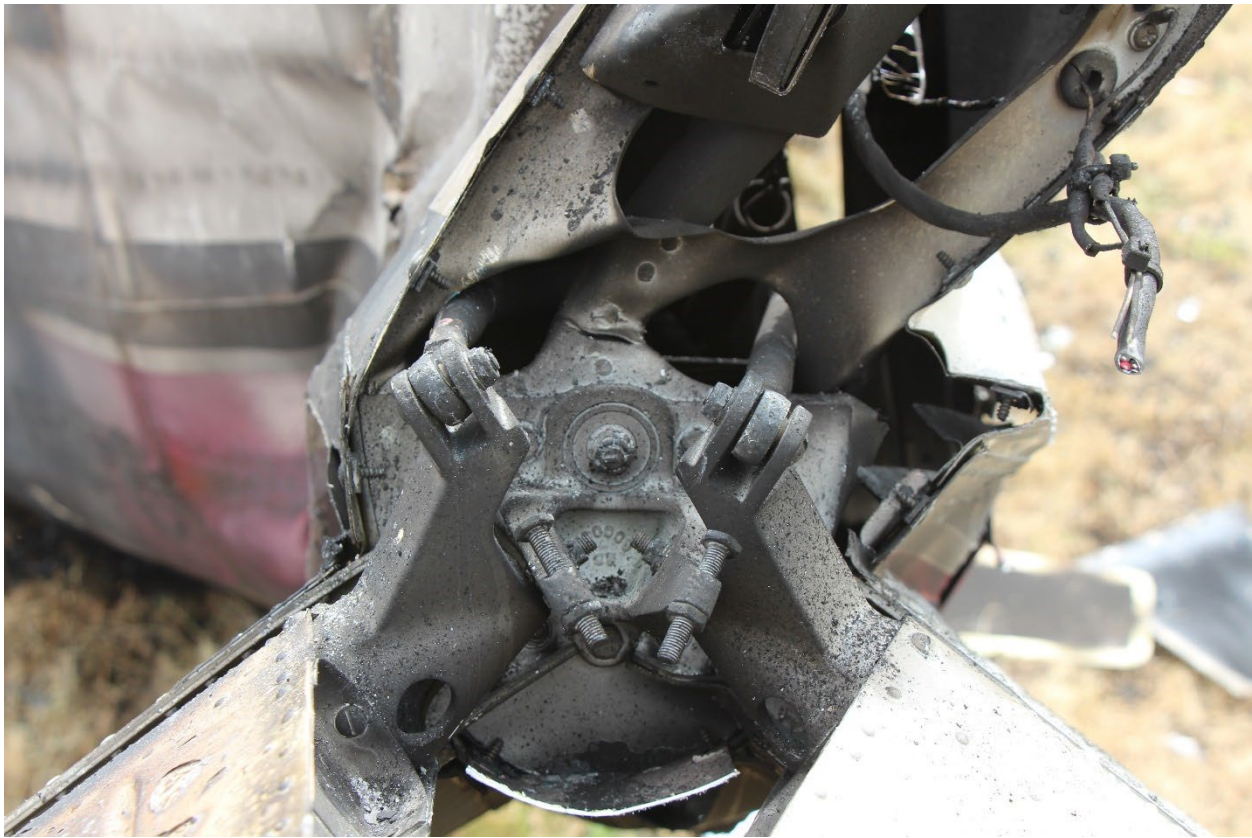
Photograph 4: Differential tail control rod attachments to rudder/elevators torque fittings
