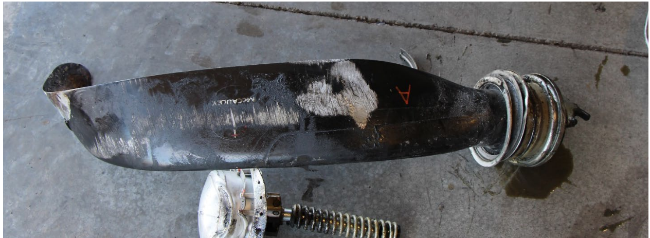
Photograph 10: Blade A with striations and tip curling
