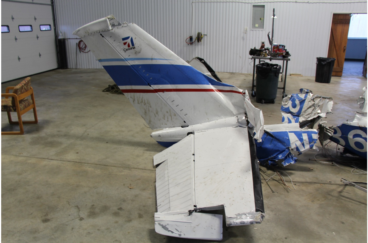
Photograph 4: Postaccident Condition of Tail Section
