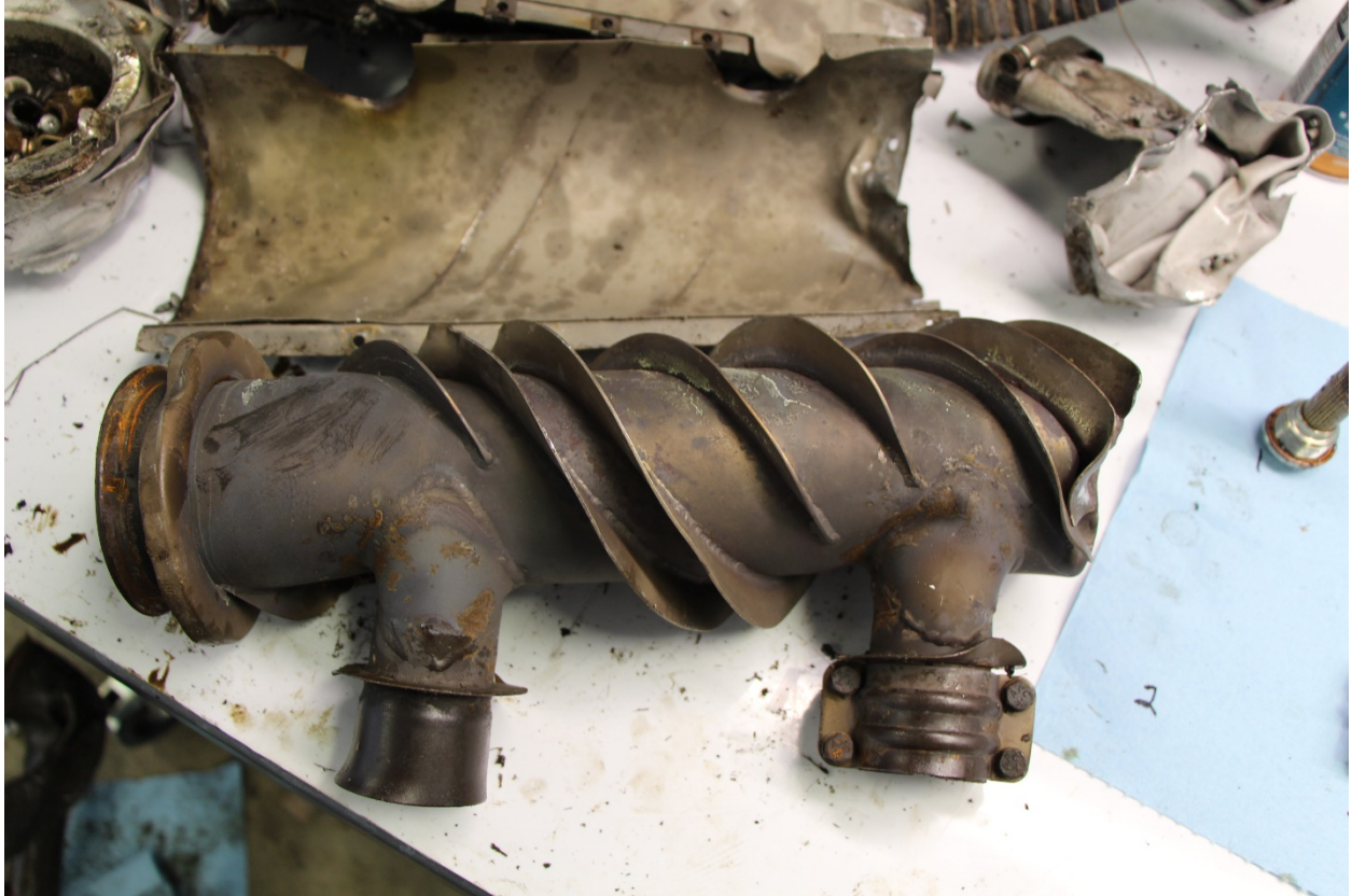
Photograph 10: Exhaust Inner Shroud
