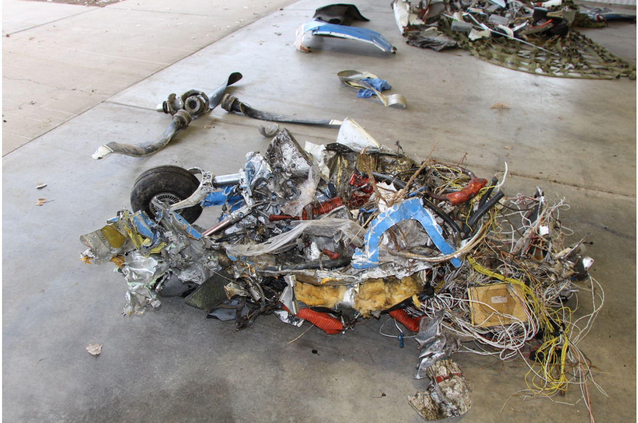
Photograph 2: Postaccident Condition of Cockpit Area and Instrument Panel
