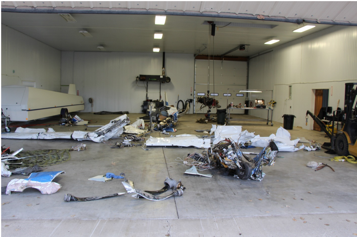
Photograph 1: Layout of Wreckage
