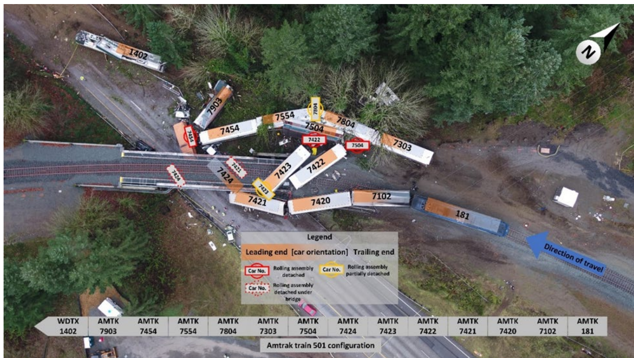
Figure 1. Overhead view of the DuPont accident site showing railcar numbers, their position in the consist, and their direction of travel. Railcar 7424 was under the overpass.
