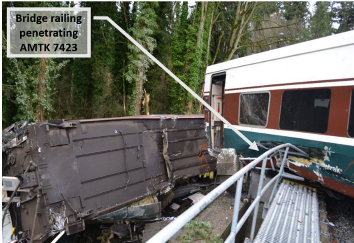
Figure 5. The bottom of railcar 7504 on the left shows no evidence of the railcar sliding sideways.
