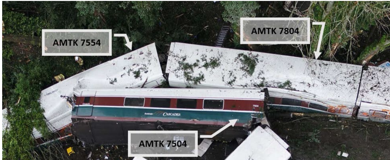
Figure 7. The right side of railcar 7504, at rest on top of railcar 7554 and alongside railcar 7804. The indentation of the roof of railcar 7804 begins just above the last window, and there are scrape marks along railcar 7804 and the trailing railcar 7303, again indicating that railcar 7504 slid backward alongside these railcars to its final resting position.
