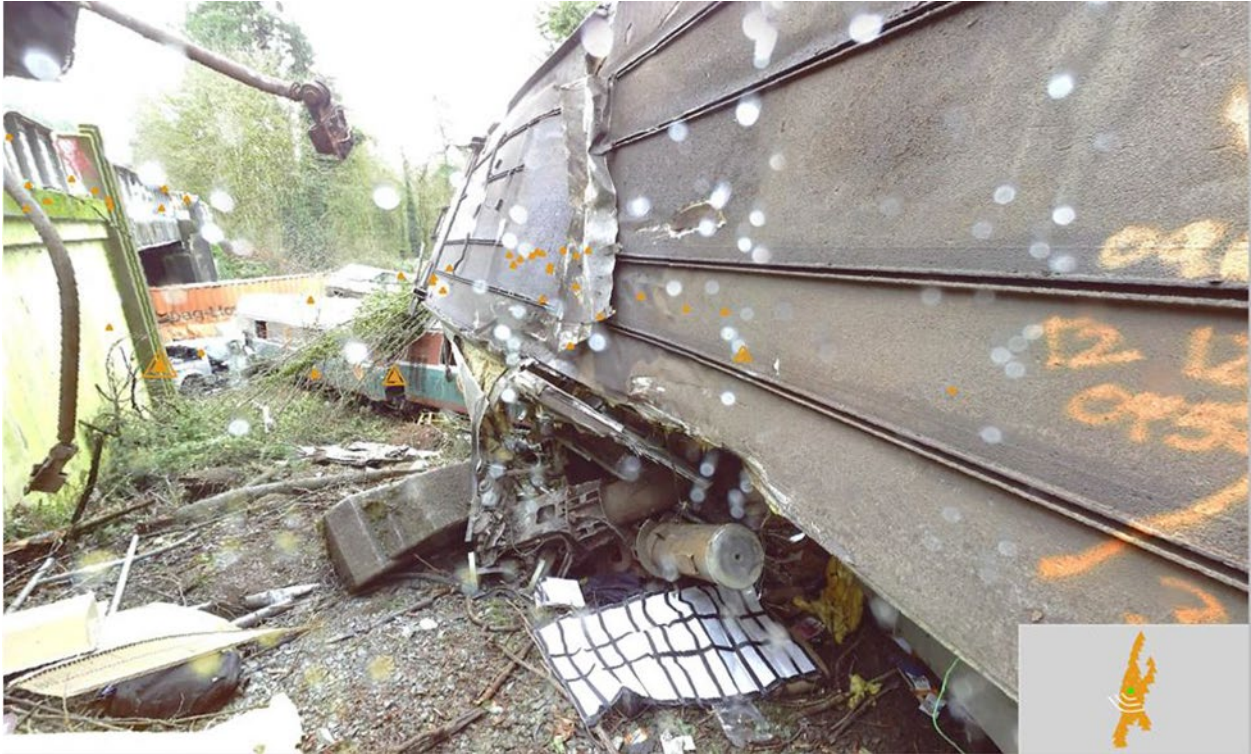
Figure 6. The bottom of railcar 7504 is on the right, looking in the opposite direction from figure 5. There are no marks to indicate the railcar slid sideways, and the bottom structure is not deformed. The detached rolling assembly from railcar 7422 is underneath railcar 7504.
