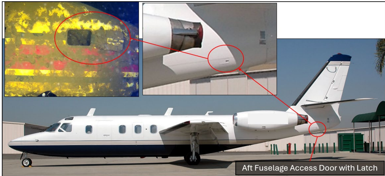
Figure 7: Exemplar airplane showing location of Aft Fuselage Access Door with latch.
