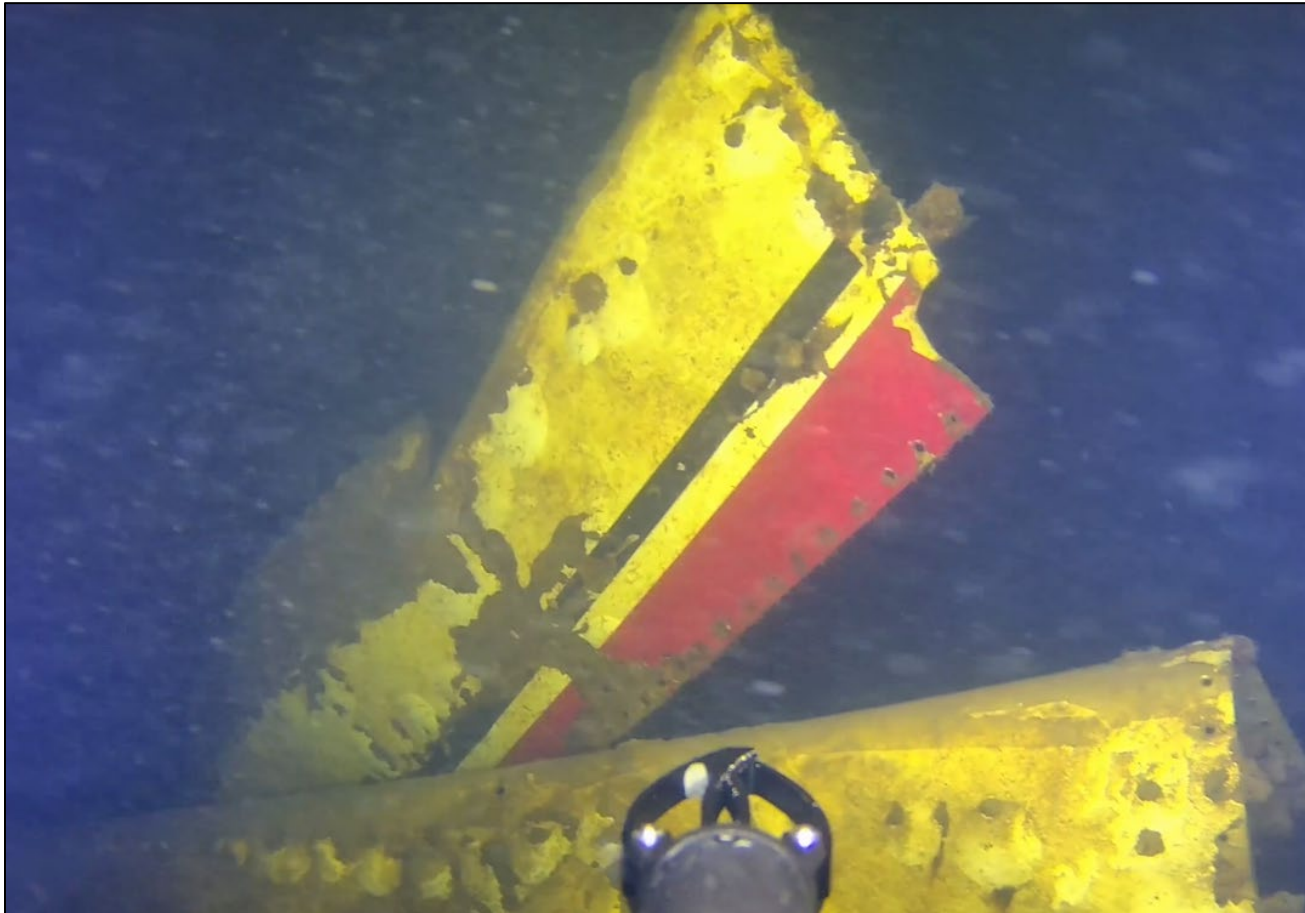
Figure 14: Additional view of paint scheme and fuselage skin matching reported picture of accident airplane.
