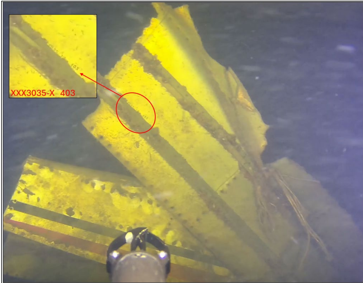
Figure 8: View of fuselage plating denoting the station location near '403' and an excerpt of Part No. '3035'.
