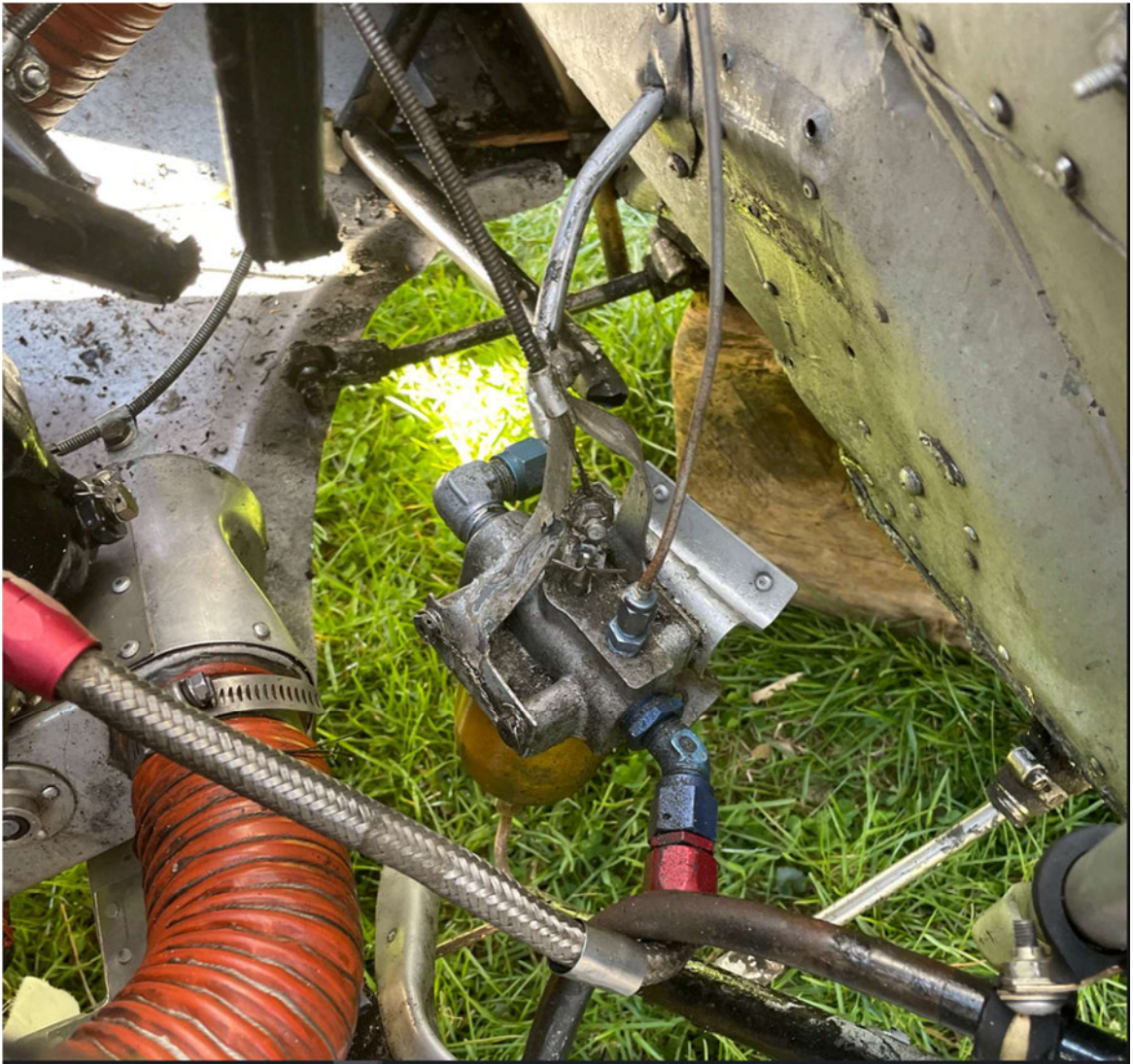
Figure 3: FAA Digital Photograph. View of the Separated Airframe Fuel Strainer. Note the Damaged Fuel Inlet Line.
