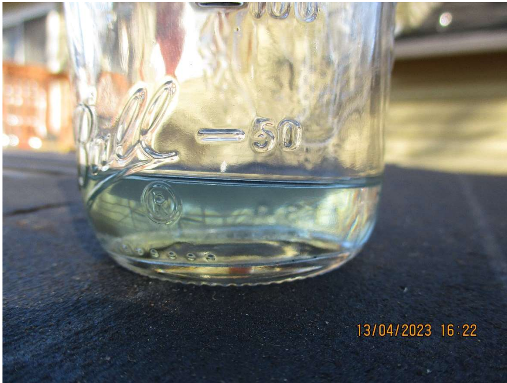
Figure 2: FAA Digital Photograph. View of the Fuel Drained From the Airframe Fuel Strainer. Note the value was about 40 milliliters.
