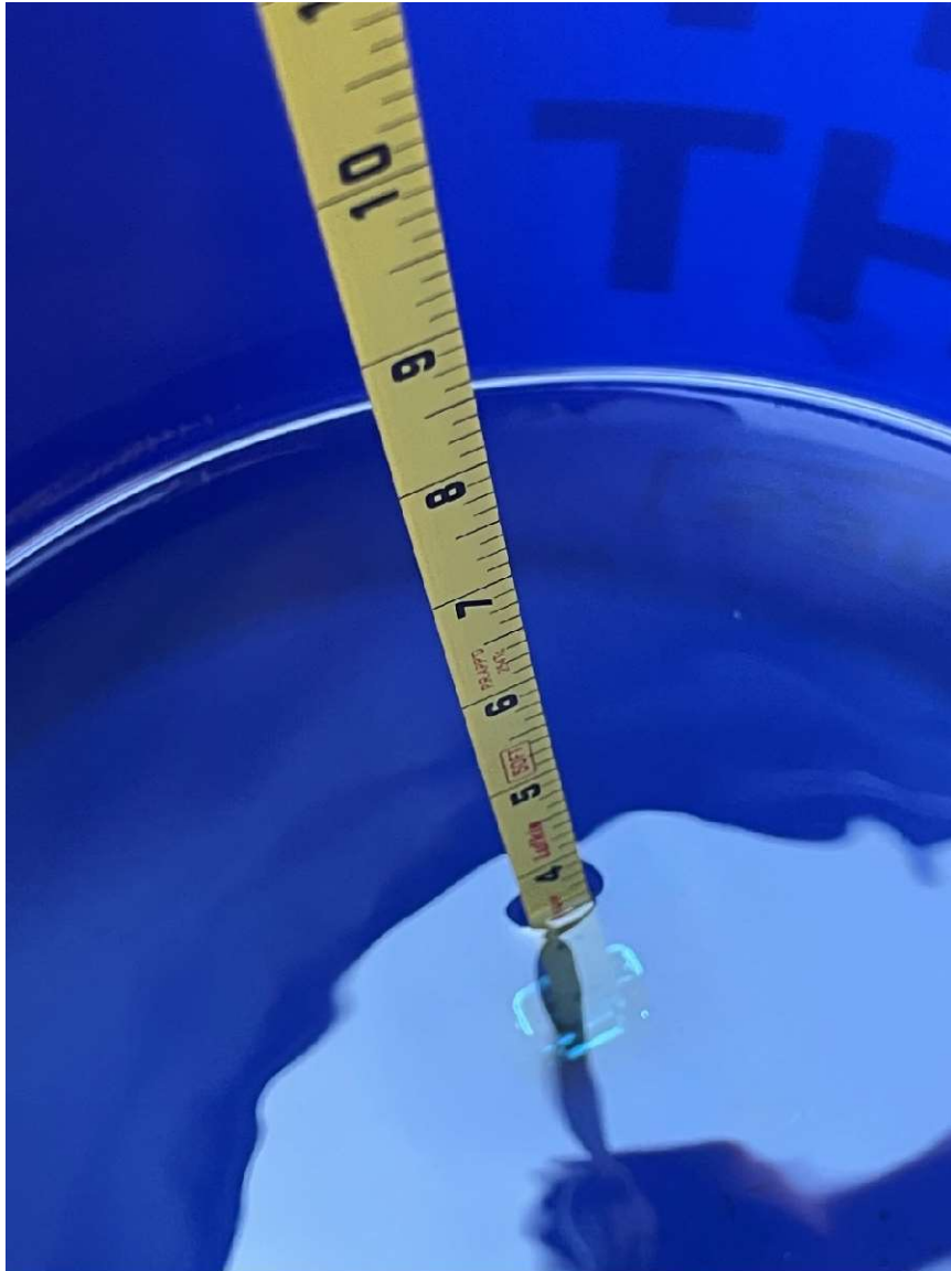
Figure 1: FAA Digital Photograph. View of the Level of Fuel Drained From the Right Wing Fuel Tank Into a 5-Gallon Bucket.
