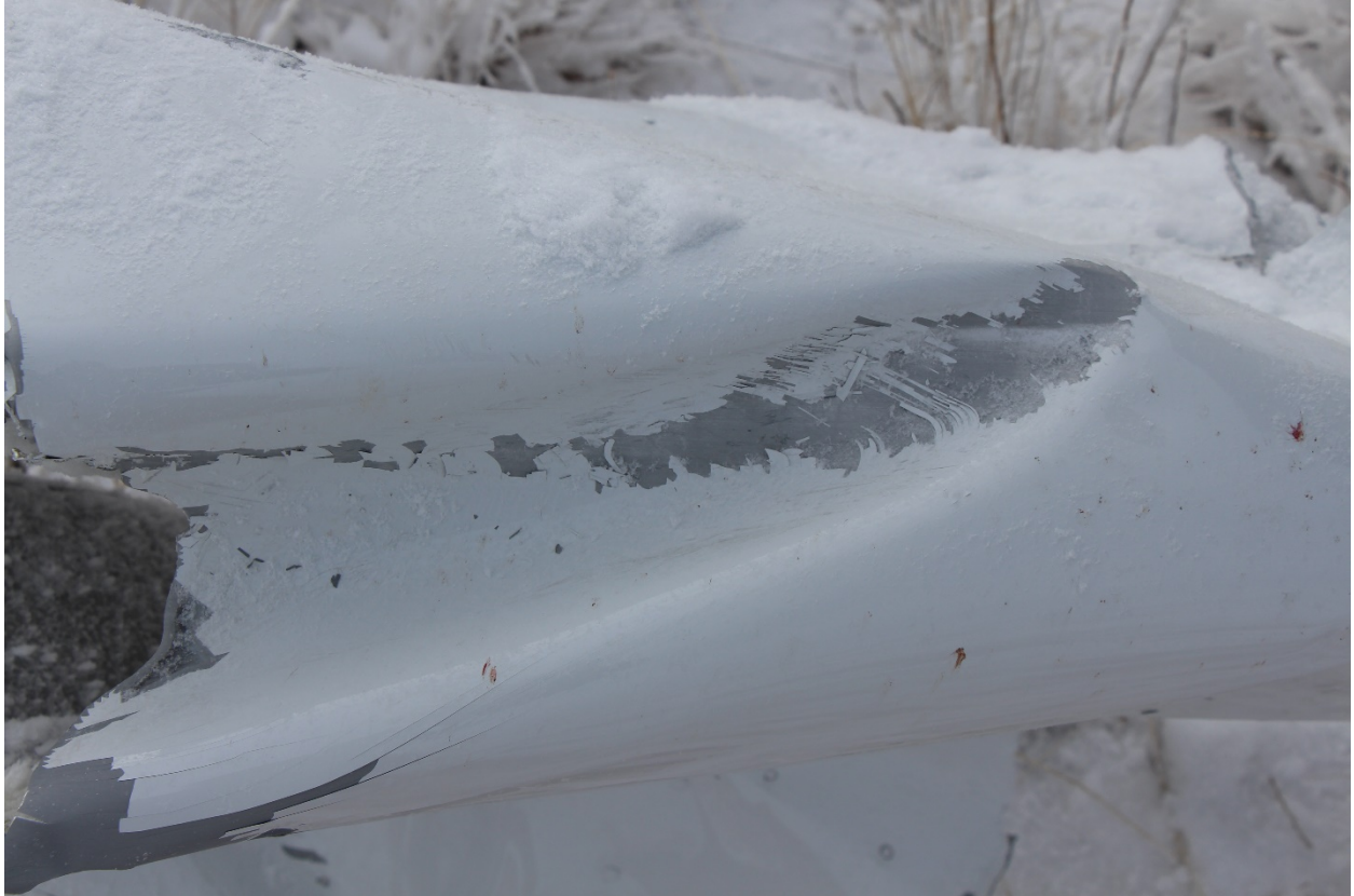
Photograph 3: Longitudinal Signature on Left Wing
