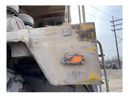
The lack of damage to the front right passenger side of the Stein dump truck indicates the truck was close to, but not on, the track when it was struck. Stated differently, if the front passenger side of the Stein dump truck extended onto the track, the damage to the truck would have been far more extensive.
