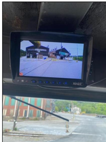
Figure 7 Example of added camera and monitor to help assist in field of vision.
