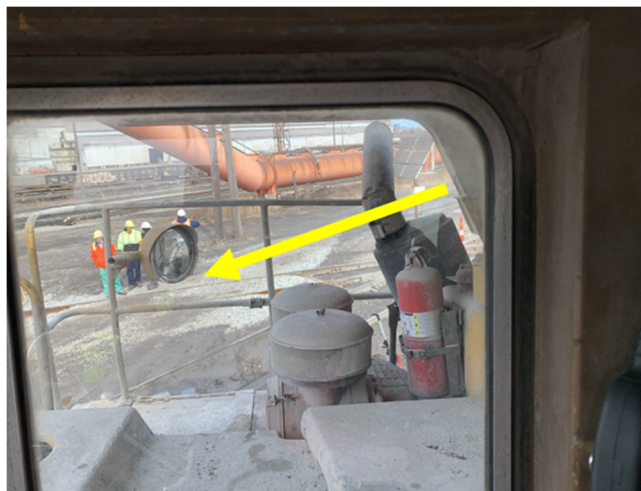
Figure 5 – Post accident re-enactment view from the Stein, LLC dump truck driver's seat with arrow added depicting angle of NS C75B106's approach path (Photo courtesy of NTSB)
