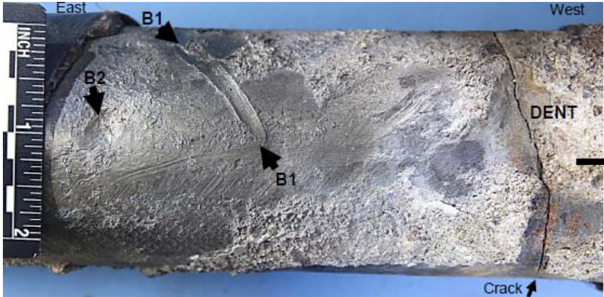
Figure 13— Showing the pipe surface after the hard deposit was removed (NTSB Materials Laboratory Factual Report 18-067)
