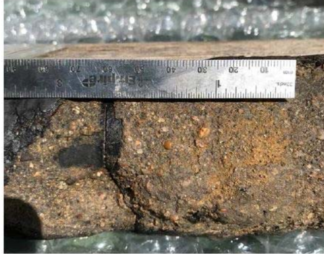
Circumferential crack in steel 2-inch-diameter pipeline.
