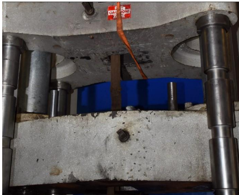
Lab setup loading the strap in simple tension
