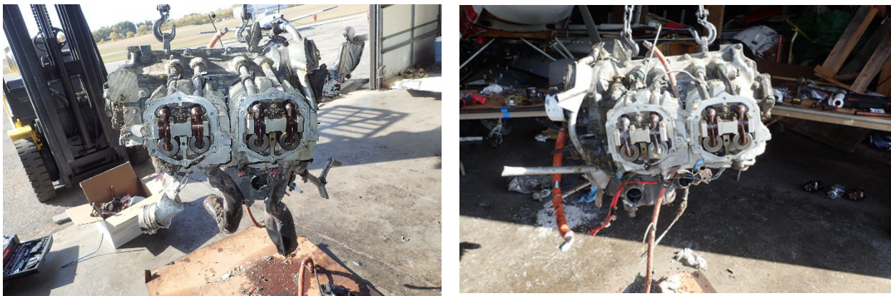
Figure 6 Engine with valve covers off.
