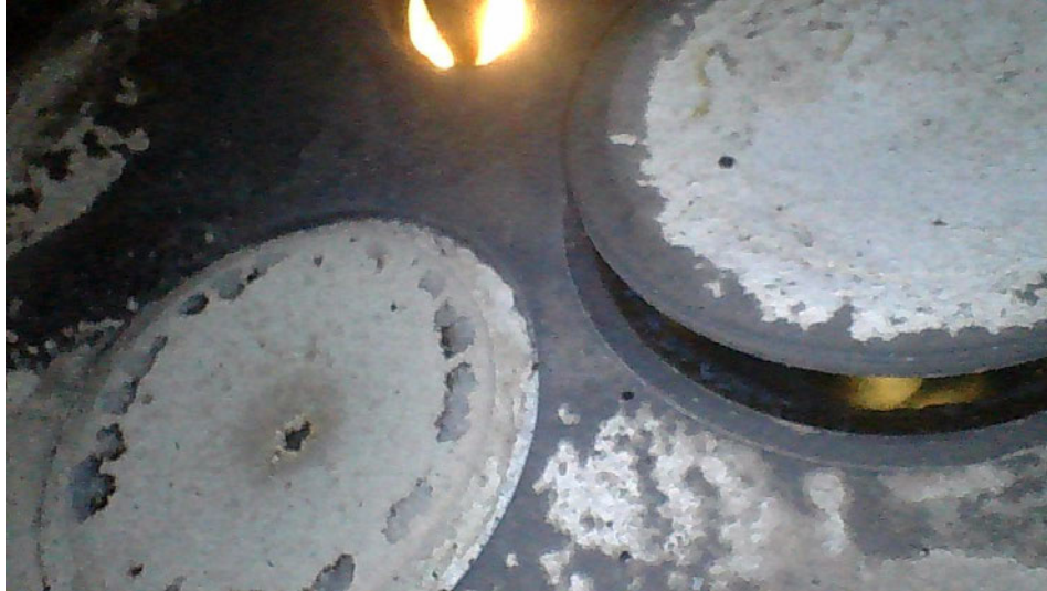
Figure 7 Borescope of No. 4 Typical of all 4 pistons, valves, and cylinders.
