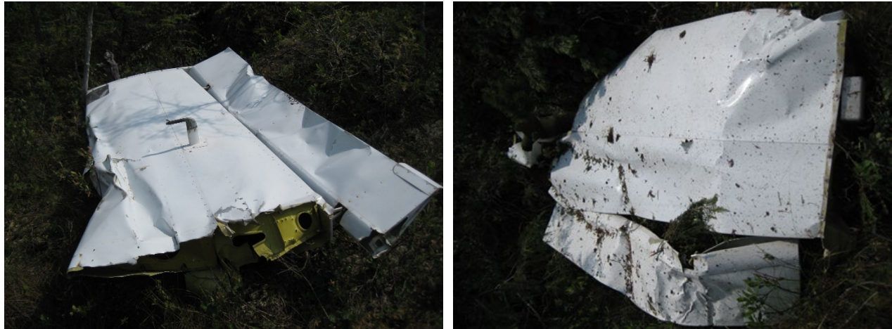
Figure 6. Underside of left wing outboard section (left) and right wing section
