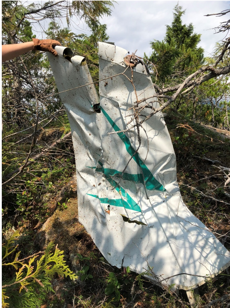
Figure 8. Vertical stabilizer and rudder
