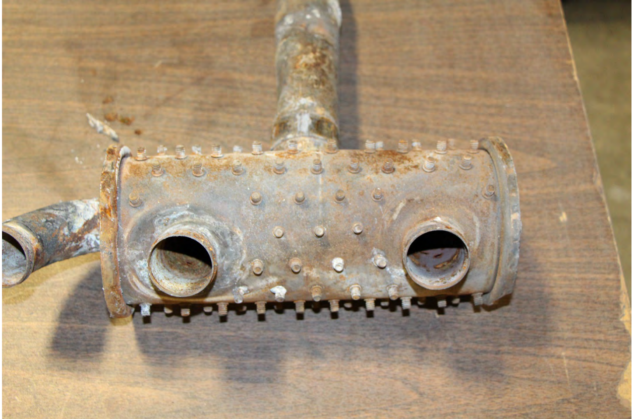
Photograph 10: Exhaust Lining to Cylinder nos. 2, 4, 6
