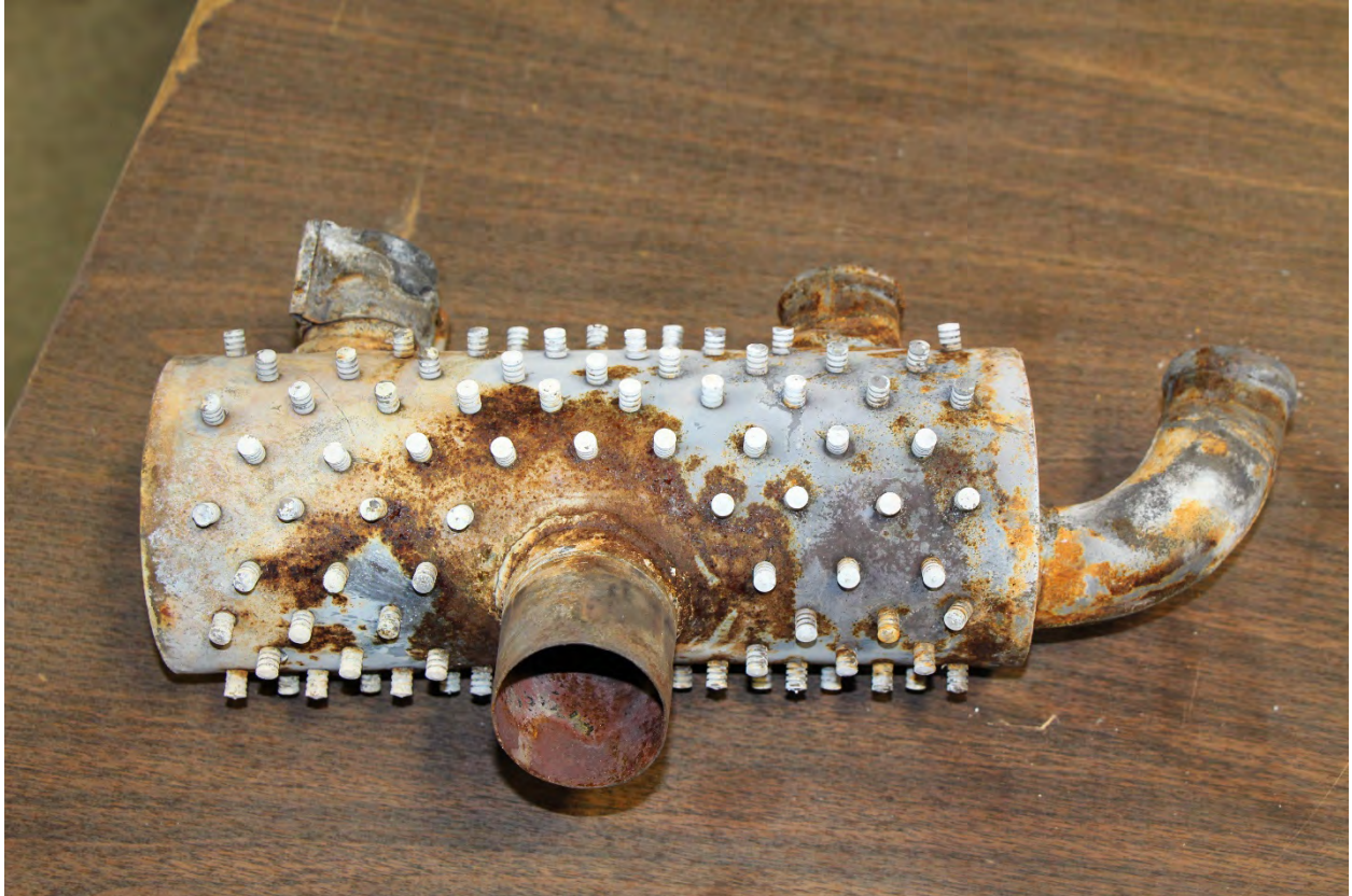
Photograph 9: Exhaust Lining to Cylinder nos. 1, 3, 5
