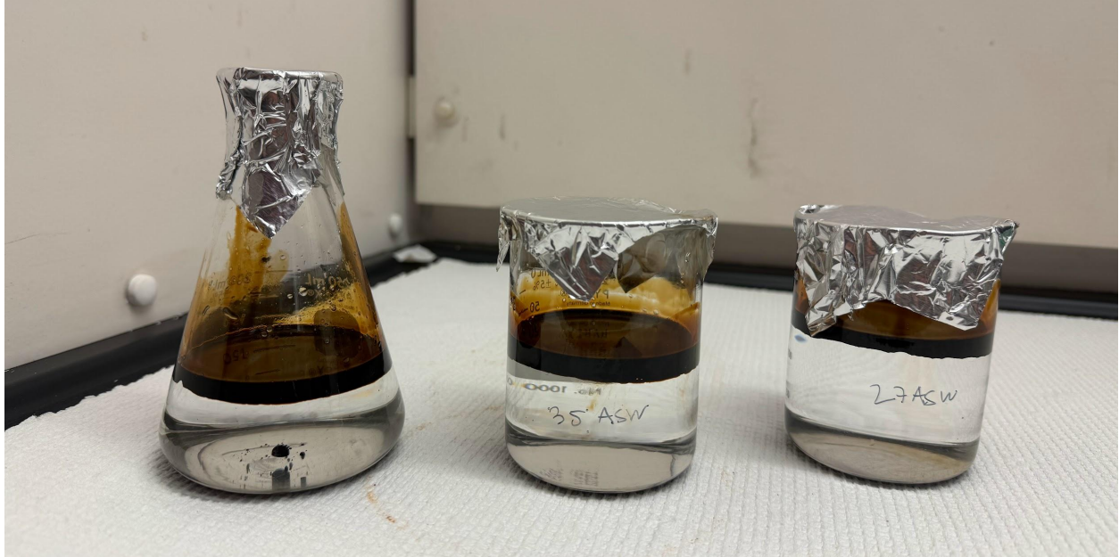
Figure 11. Laboratory tests with the source oil and different salinities and flask types (Erlenmeyer flask on the left, wide-mouth beakers in center and right).
