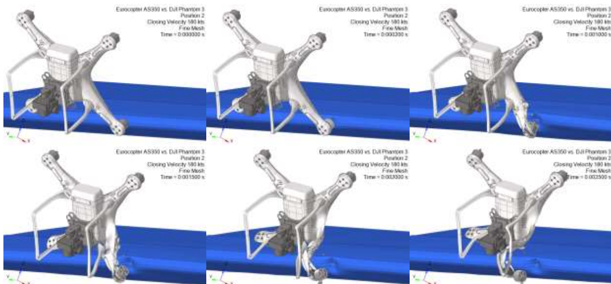
Figure 2.12 T5 Impact Kinematics Progression – 180 kts in Position 2 With Fine HSLE Skin Mesh
