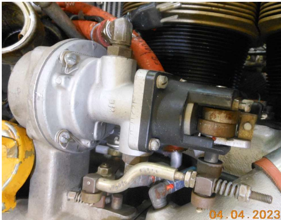
Photo #9 – Variable Absolute Pressure Controller
