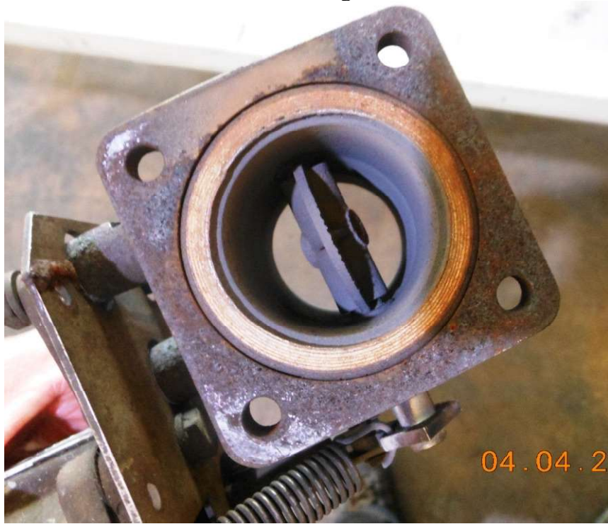
Photo #8 – Wastegate valve
