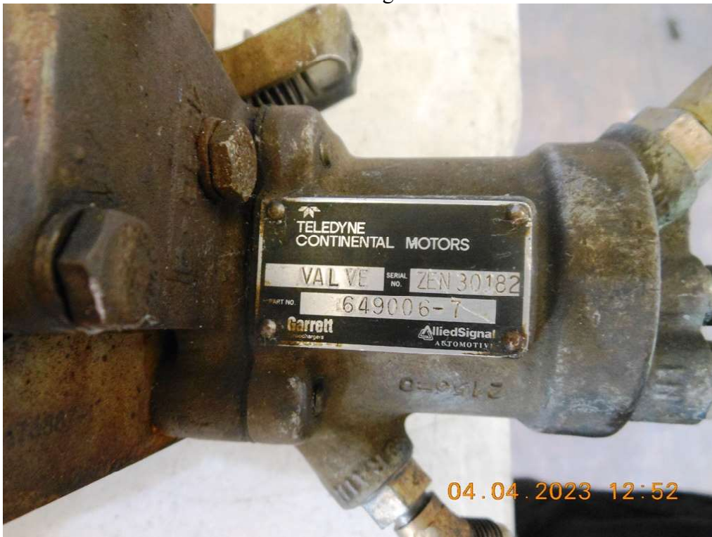
Photo #7 – Wastegate actuator
