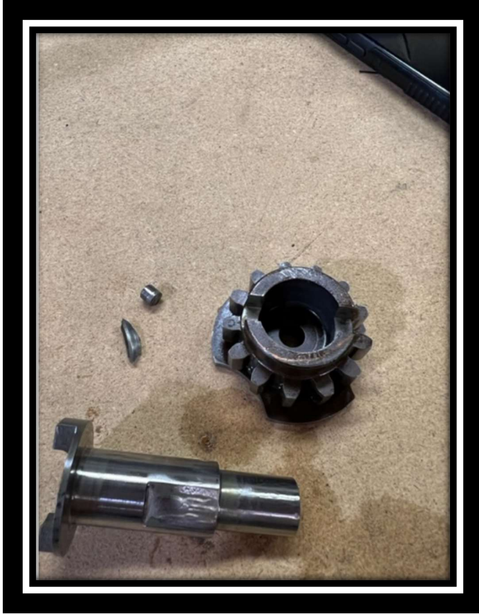
Figure 4 Center Crankshaft Gear, Oil Pump Drive shaft, Sheared Gear Alignment Pin and Material from damaged Crankshaft machined Gear Boss.
