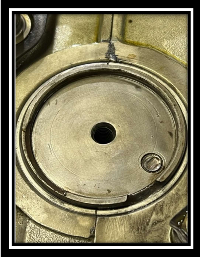
Figure 3 Close Up View of Gear Alignment Pin Sheared off and Missing Crankshaft Machined Gear Boss.
