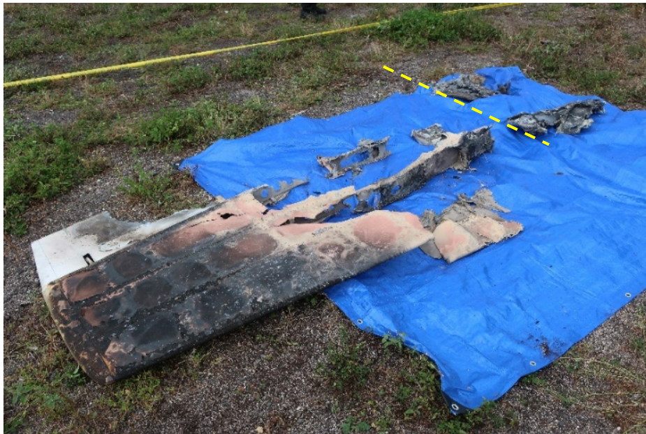
Figure 48. Partial reconstruction as seen from the front right. The yellow line denotes the centerline of the tail of the fuselage. The aft left spar stub fragment (Figure 50) is not in this photo. (Photo from: Swaim)
