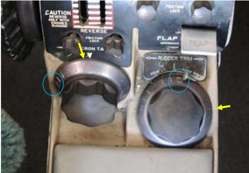
Figure 20. As-found position of aileron trim (left knob) in full left wing down orientation after the 2016 accident and of the rudder trim knob (right). The center of graduated adjustment scales in each have rectangular markings which are circled, with five lines to either side. The last adjustment marking from the right can be seen at the top of the aileron knob. A corresponding arrow shows the equivalent mark on the rudder knob as an example. (Photo from: Textron Report ASI-16-CF, taken August 11, 2016)
