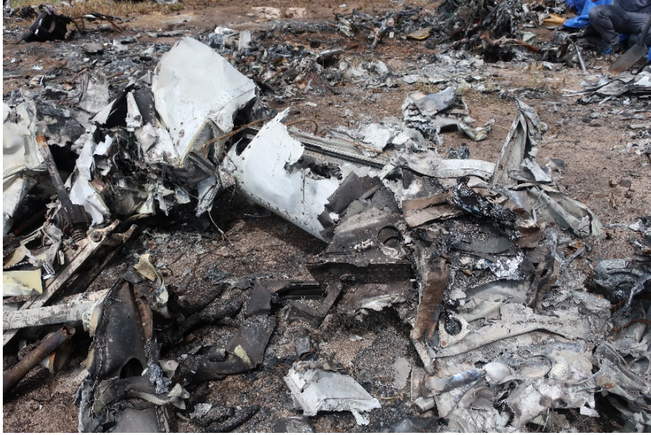
Figure 39. The remaining portion of the inboard left wing leading edge, from between the nacelle and fuselage. (Photo from: Swaim)
