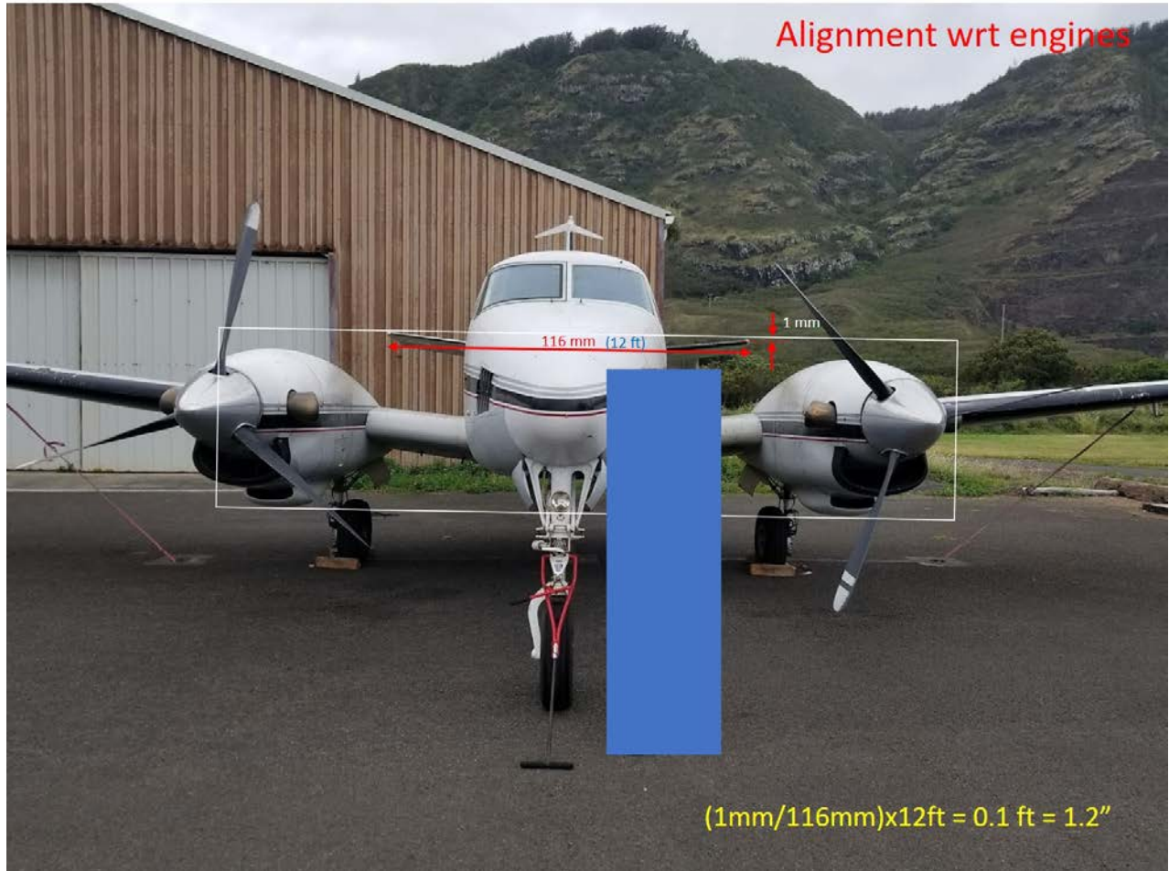
Figure 9. Front view of airplane, showing alignment measurements. (Photo from: Skinner)
