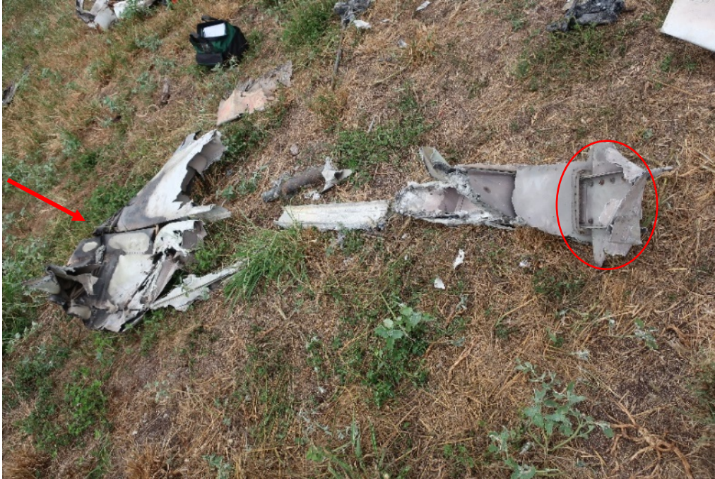
Figure 53. Fragments of the rear spar from the fuselage bulkhead (oval) to the caps of the vertical stabilizer and rudder (arrow).
