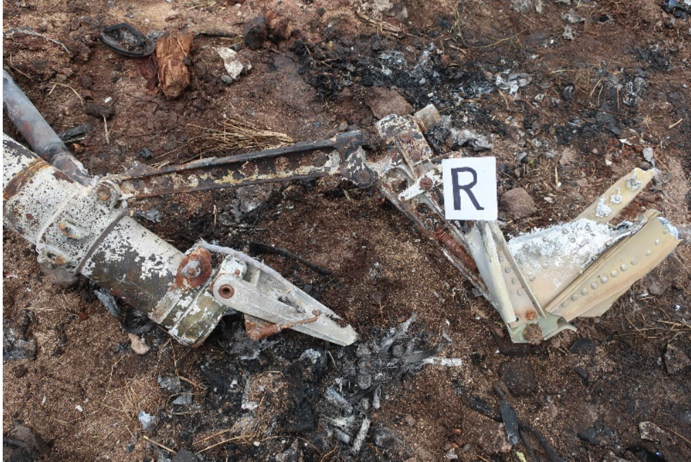
Figure 57. Right main landing gear strut and lock assembly. (Photo from: Swaim)
