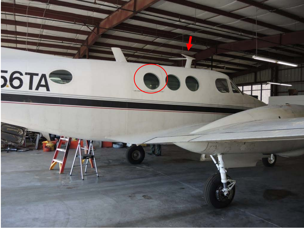
Figure 27. Arrow points to antenna shown in following photo. Oval denotes emergency exit. (Photo from: Textron Report ASI-16-CF, taken August 11, 2016)
