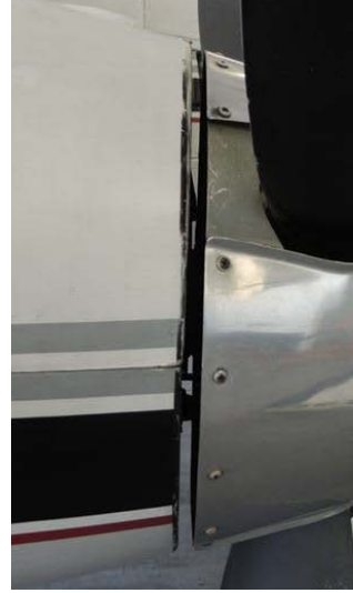
Figure 16B. Gap between right spinner and cowl, showing parallel edges. (Photo from: Textron Report ASI-16-CF, taken August 11, 2016)
