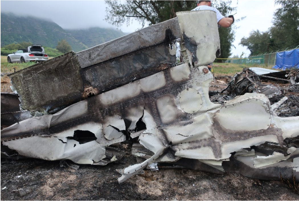
Figure 33. Bottom surface of remaining left aileron and wing. (Photo from: Swaim)
