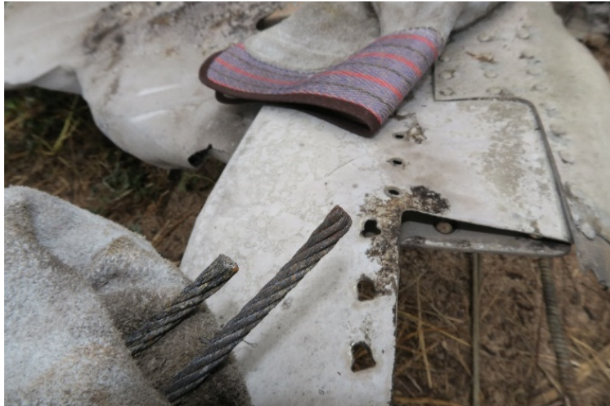
Figure 77. Post fire cut right wing aileron control cables. (Photo from: Textron)
