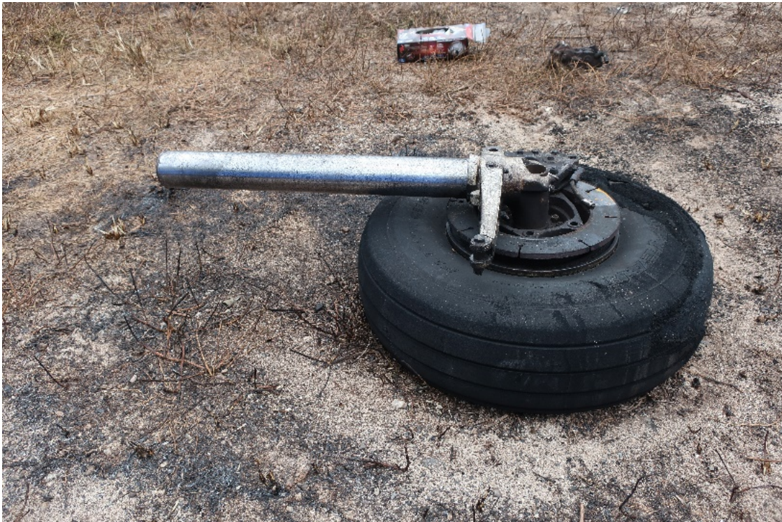
Figure 56. Left main landing gear with inner strut, separated from outer strut and found to east of the majority of the debris. (Photo from: Swaim)
