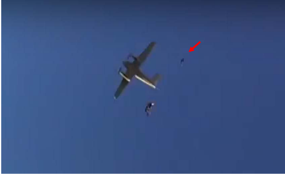
Figure 2. Still image from skydiver Achal Asawa video during freefall shows missing right horizontal stabilizer and elevator assembly (arrow) and another skydiver.
