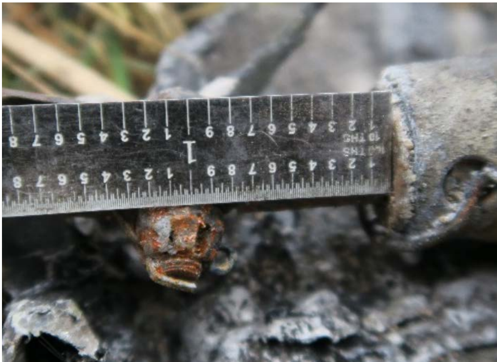
Figure 76. Right pitch control trim extension. (Photo from: Textron)
