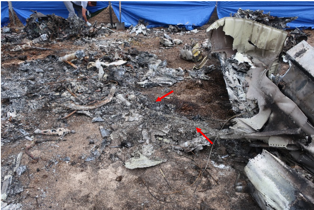
Figure 38. Arrows show remnants of left wing rear spar between wing at right and nacelle at upper left, where engine was found. (Photo from: Swaim)
