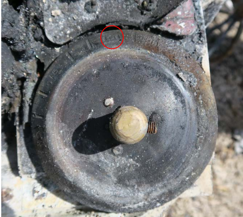
Figure 86. Rudder trim control knob with center “0” marking circled. (Photo from: Textron)
