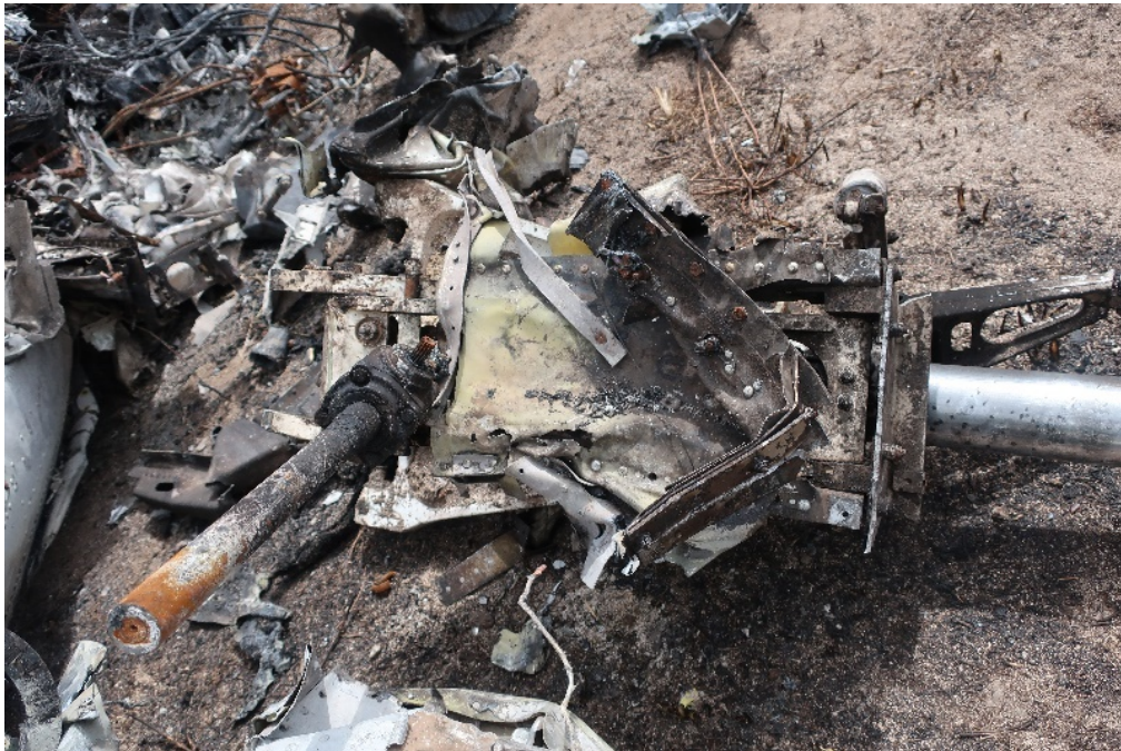
Figure 58. Top of the nose landing gear assembly with the box fragments bent aft toward the tire.
