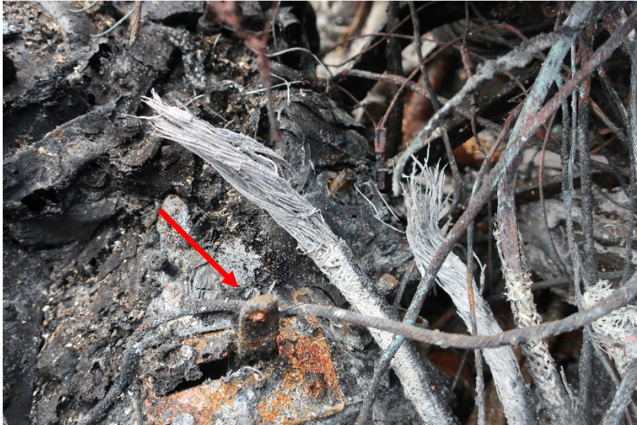
Figure 89. Arrow points to remnant of flap handle.
