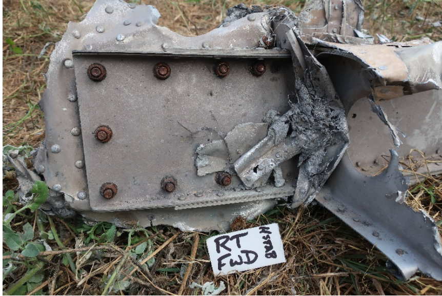
Figure 51. Right horizontal stabilizer forward spar stub bolted to a remnant of the aft fuselage bulkhead. (Photo from: Swaim)
