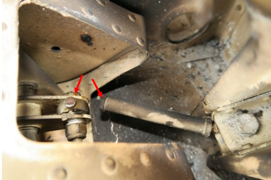
Figure 81. Right aileron tab anti-servo rod assembly with red arrows indicating the fracture surfaces (Photo from: Textron)
