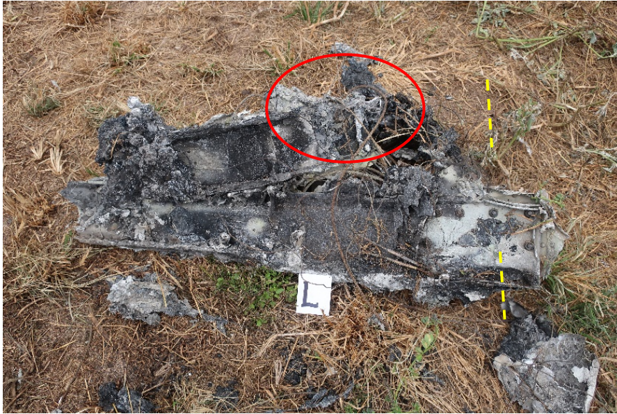
Figure 49. Left horizontal stabilizer bent in half with the oval denoting the forward spar stub bolted to a remnant of the aft fuselage bulkhead. The yellow lines denote the side of the aft fuselage, showing small amounts of the bulkhead remaining attached to the spar stub. (Photo from: Swaim)
