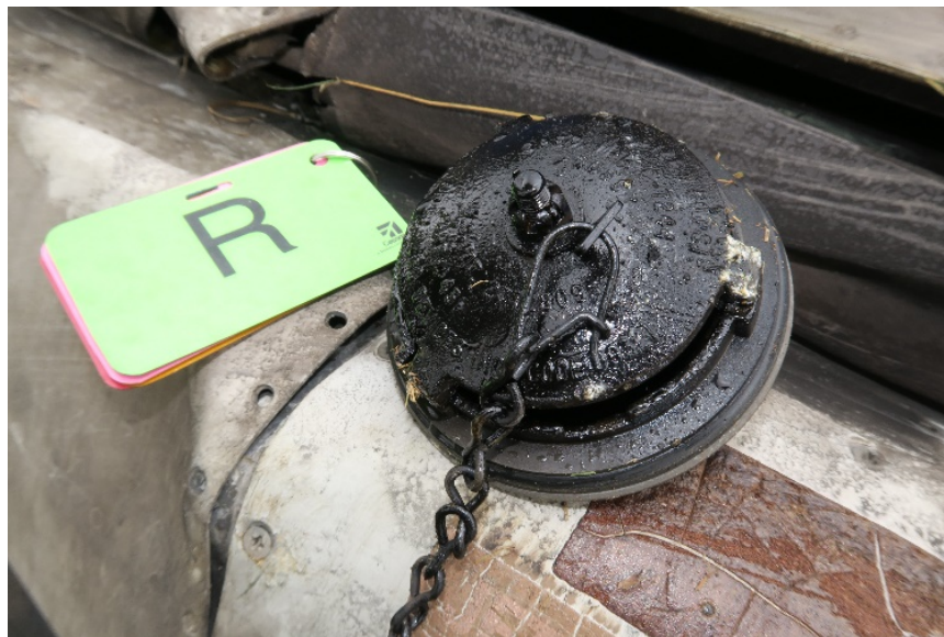
Figure 60. Right wing fuel cap with fire residue. (Photo from: Textron)
