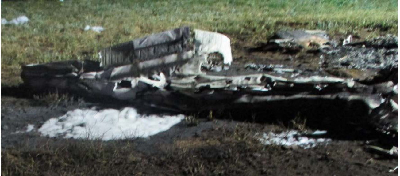
Figure 31. Left wing in initial night photo, seen oriented with the leading edge downward prior to victim recovery. (Photo from: FAA)
