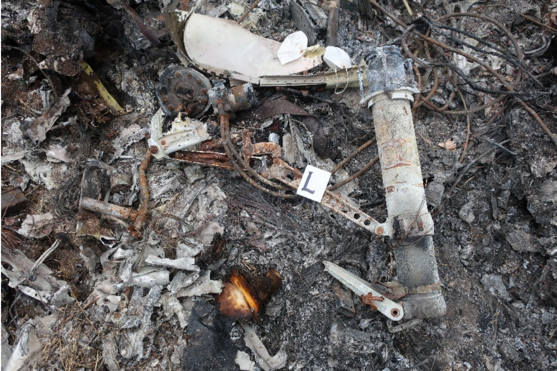
Figure 55. Left main landing gear strut and lock assembly. (Photo from: Swaim)
