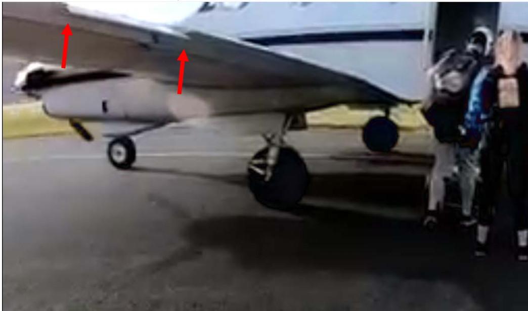
Figure 19. The extent of left aileron trim tab deflection is clearly visible between the arrows while loading for the flight prior to the accident. (Video from: Public)
