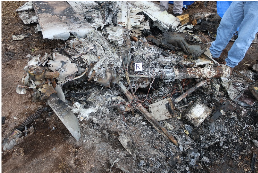
Figure 43. Right nacelle with outboard wing panel beyond. The main landing gear strut cylinder is the horizontal tube extending from the “R” to the person’s foot. The inner portion of the landing gear strut with the tire was partially beneath the airport perimeter fence. (Photo from: Swaim)
