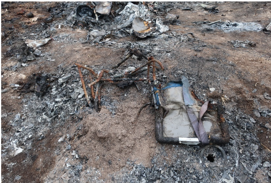
Figure 64. Remnants of pilot seat. The circular item below the seat is the left propeller hub. (Photo from: Swaim)
