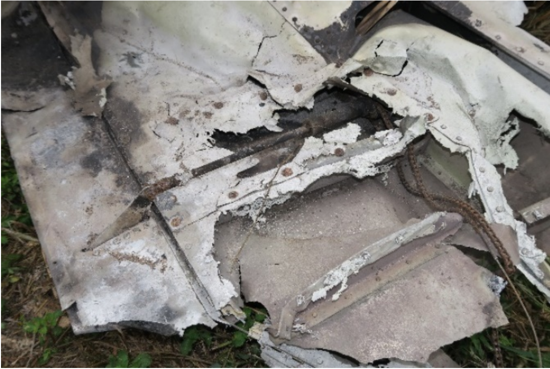
Figure 87. Rudder and trim remnants with exposed trim actuator. (Photo from: Textron)
