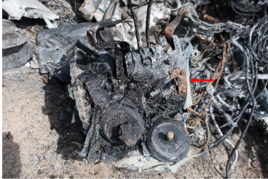
Figure 83. Cockpit control pedestal with aileron trim knob to left and rudder trim knob to right. Arrow points to flap handle in up/retracted position. (Photo from: Swaim)
