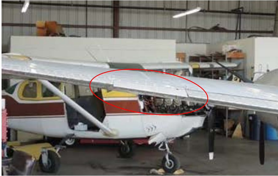
Figure 17. Deflection of aileron trim tab on left wing photographed during inspection after 2016 loss of horizontal stabilizer. (Photo from: Textron Report ASI-16-CF, taken August 11, 2016)
