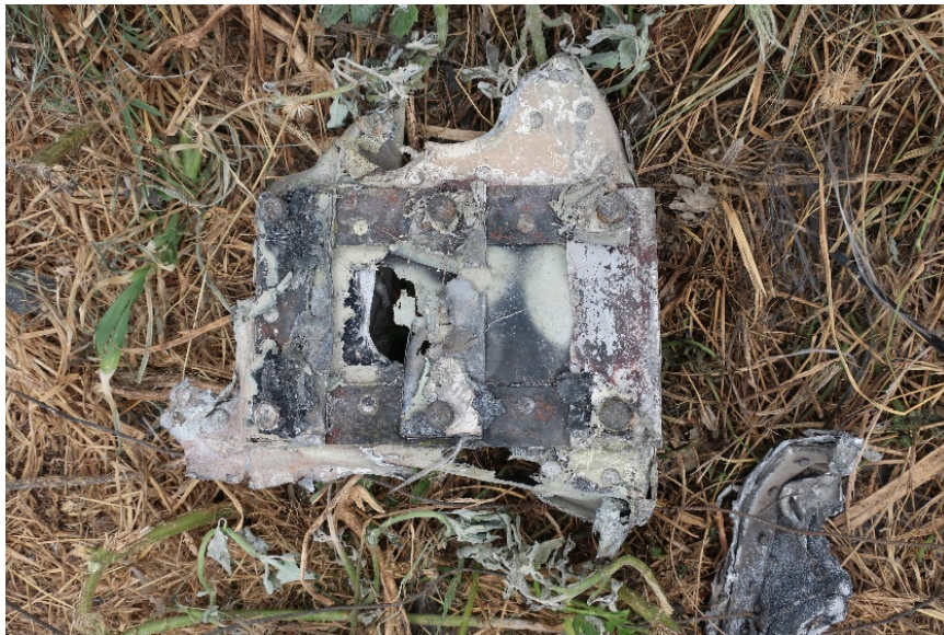
Figure 52. Attachment of right horizontal stabilizer rear spar stub to airplane bulkhead. (Photo from: Swaim)
