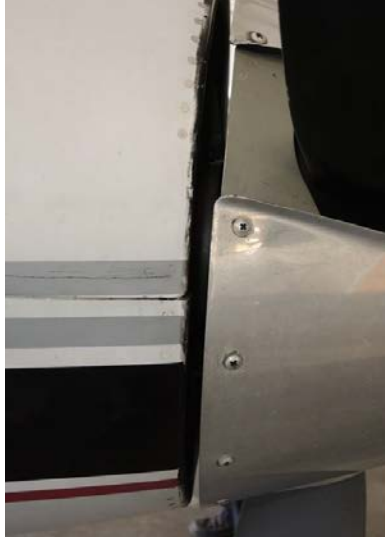
Figure 16A. Gap between left spinner and cowl, showing edges not parallel with propeller oriented downward. (Photo from: Textron Report ASI-16-CF, taken August 11, 2016)
