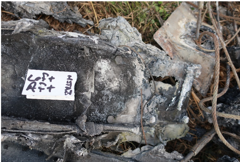
Figure 50. Left horizontal stabilizer aft spar stub remnant bolts which remained attached to a fragment of the bulkhead. (Photo from: Swaim)
