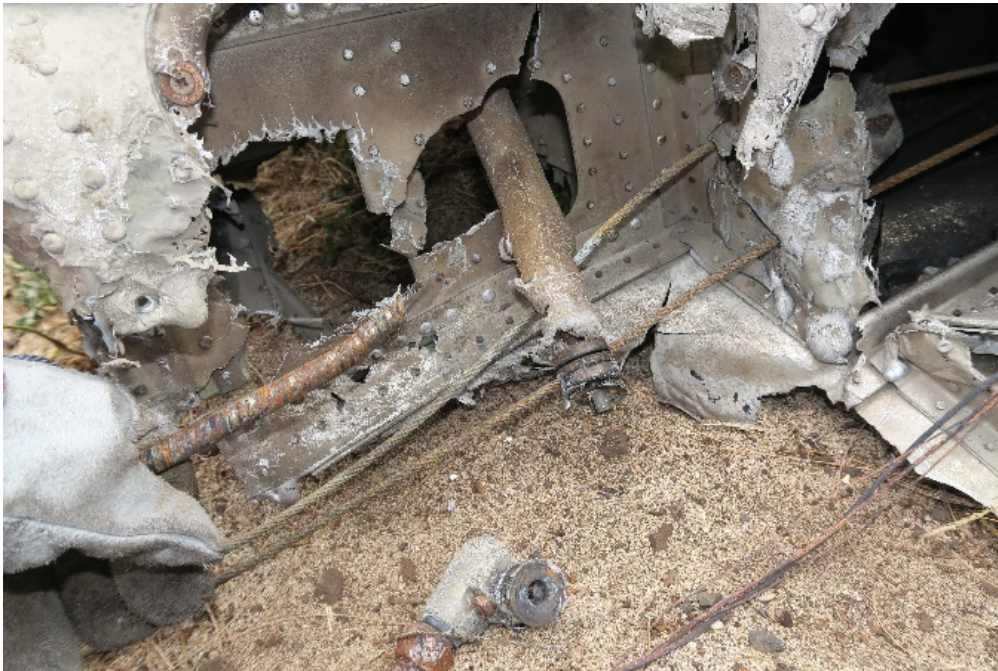
Figure 91. Broken outboard right flap actuator. (Photo from: Textron)
