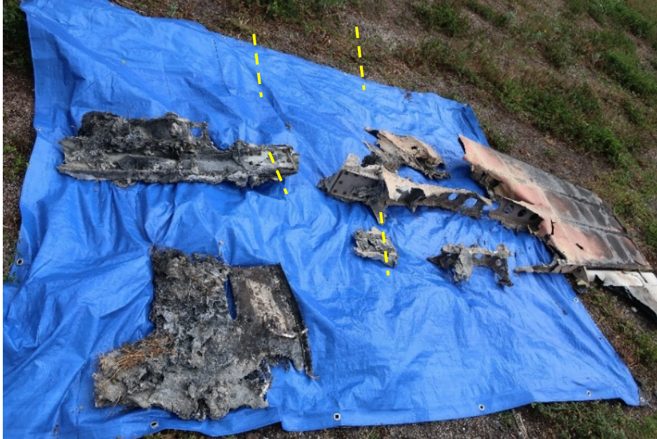
Figure 47. Partial reconstruction of horizontal stabilizers and elevators, with left toward the left and right toward the right. The yellow lines denote the relative sides of the fuselage. The aft left spar stub fragment (Figure 50) is not in this photo. (Photo from: Swaim)
