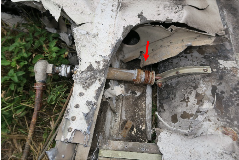
Figure 92. Right flap actuating assembly extension indicated by arrow. (Photo from: Textron)
