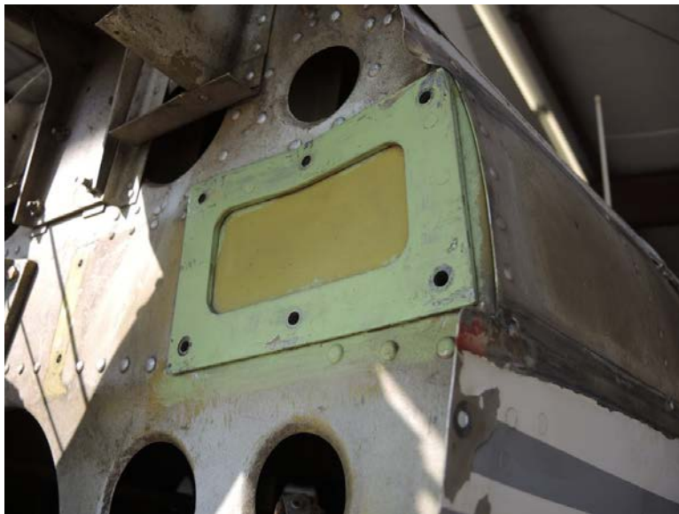
Figure 6. Closer view of the bent attachment which the right HSTAB attached to. (Photo from: Textron Report ASI-16-CF, taken August 11, 2016)
