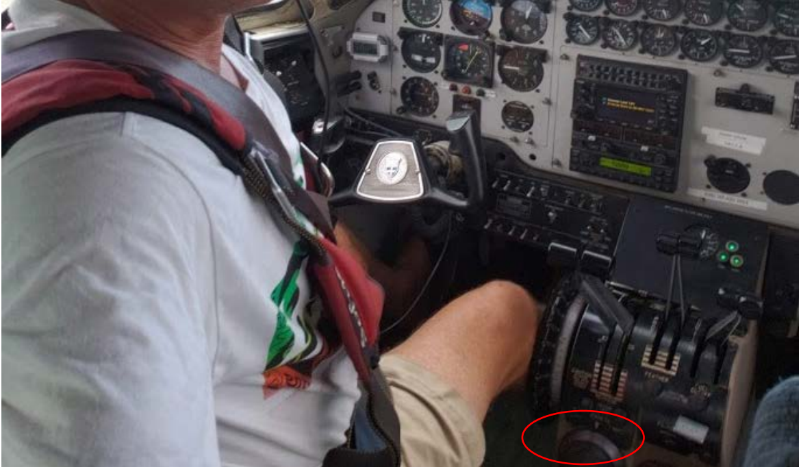
Figure 21A. This March 7, 2018 photo of a pilot recorded the aileron trim (left knob) in full left wing down orientation. (Photo from: Skinner)
