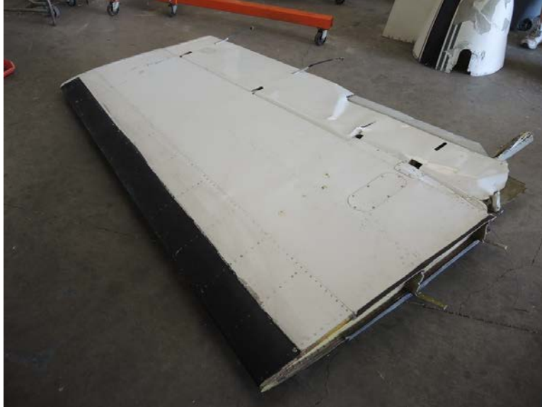
Figure 7. The damaged right HSTAB. (Photo from: Textron Report ASI-16-CF, taken August 11, 2016)
