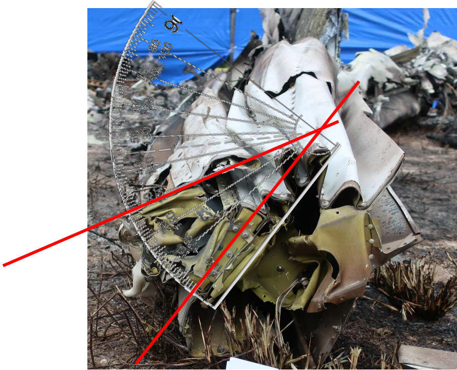
Figure 36. Crush line (upper red line) of the upper leading edge as measured to the vertical center of the wing spar (lower red line) at wing tip. (Photo from: Swaim)
