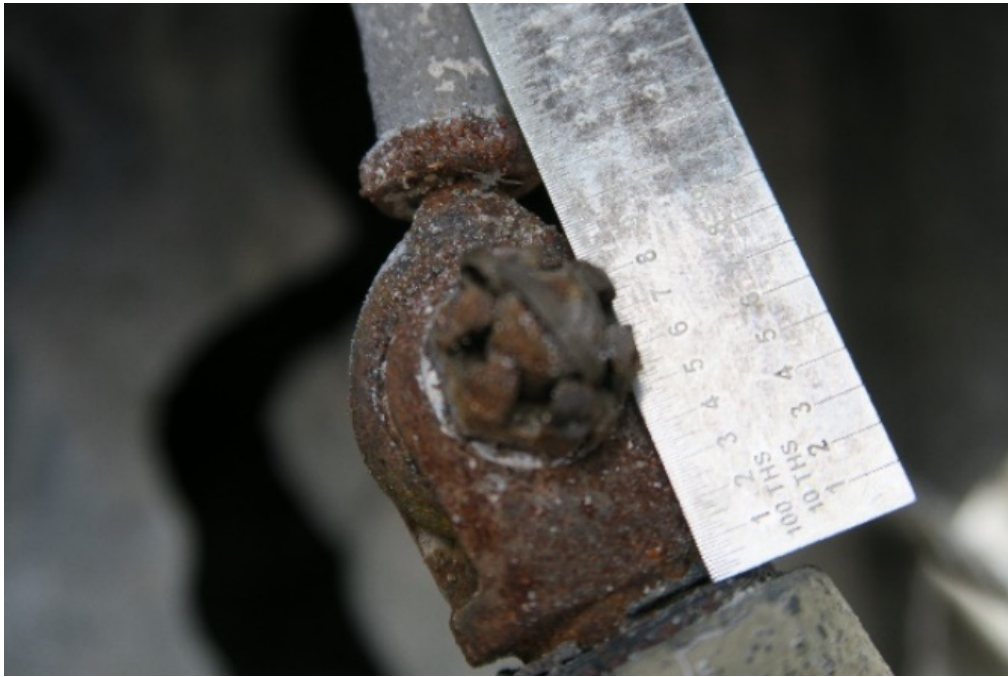
Figure 85. The aileron trim mechanism in the left wing was found extended 0.65 inches, corresponding with the position of the cockpit knob. (Photo from: Textron)
