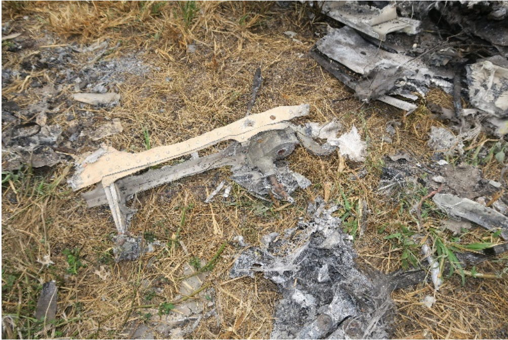
Figure 75. Right pitch control trim drum on fragment of horizontal stabilizer spar. (Photo from: Textron)
