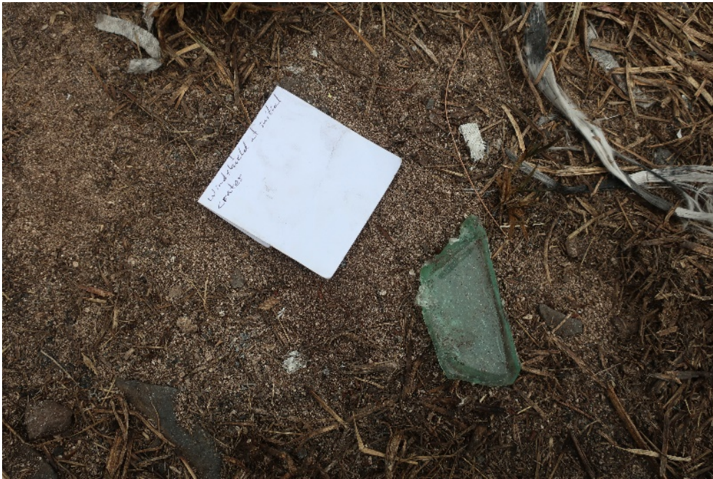
Figure 25. Windshield fragment at initial impact location. (Photo from: Swaim)
