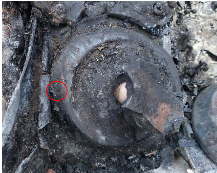
Figure 84. Closer view of aileron trim knob with center "0" marking circled. (Photo from: Textron)
