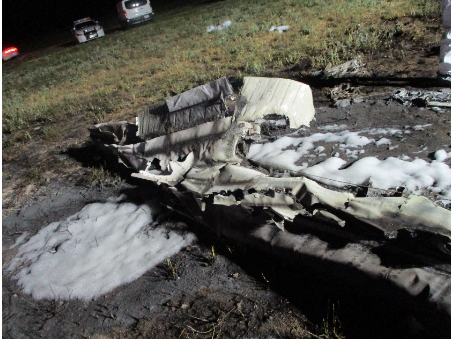
Figure 23. Left outboard wing, leading edge down. (Photo from: FAA)
