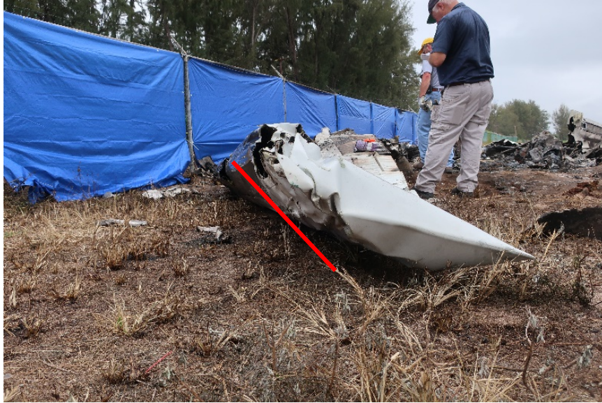
Figure 42. Right wing tip with added crush line. (Photo from: Swaim)
