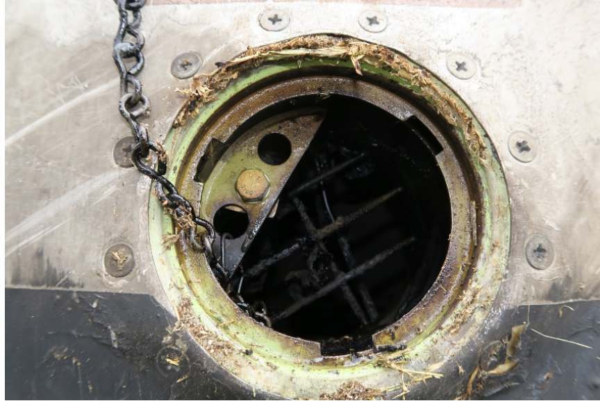
Figure 61. Interior of right fuel tank after removal of cap. (Photo from: Textron)
