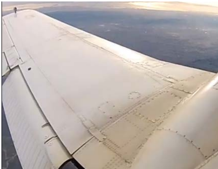
Figure 11. Pre-2016 accident photo showing lack of wrinkles and smooth transition across the outboard section of the forward wing spar. (Still image from video posted to: www.Gurustunts.com )
