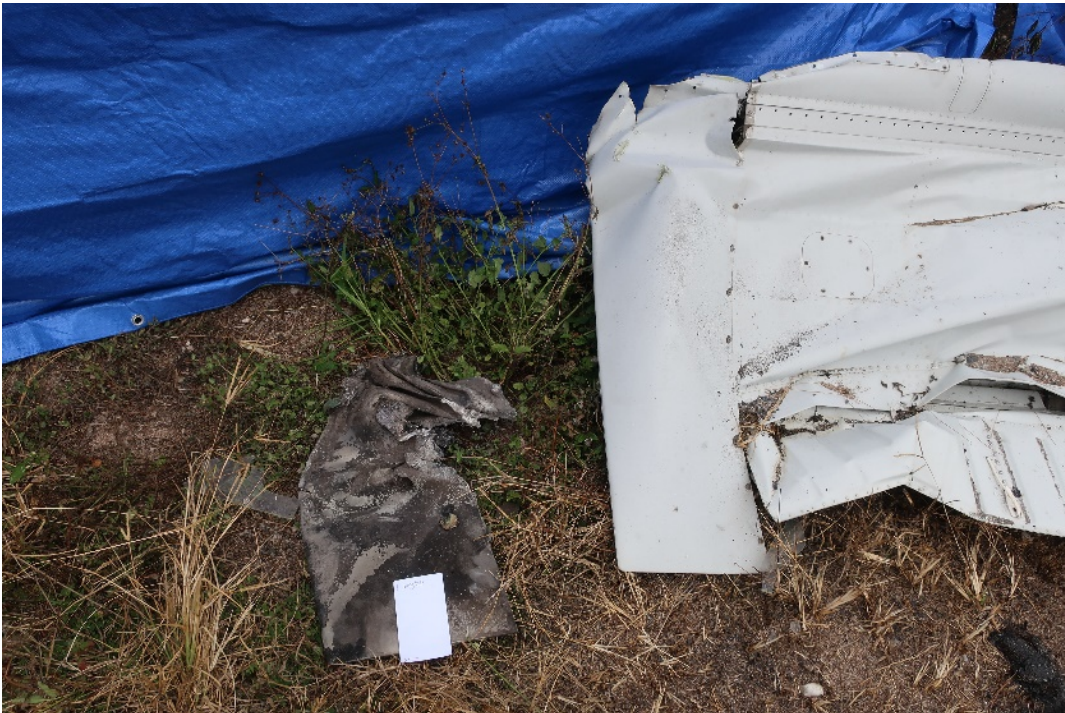
Figure 34. Burned and crushed left wing tip placed next to the tip of the right wing. (Photo from: Swaim)
