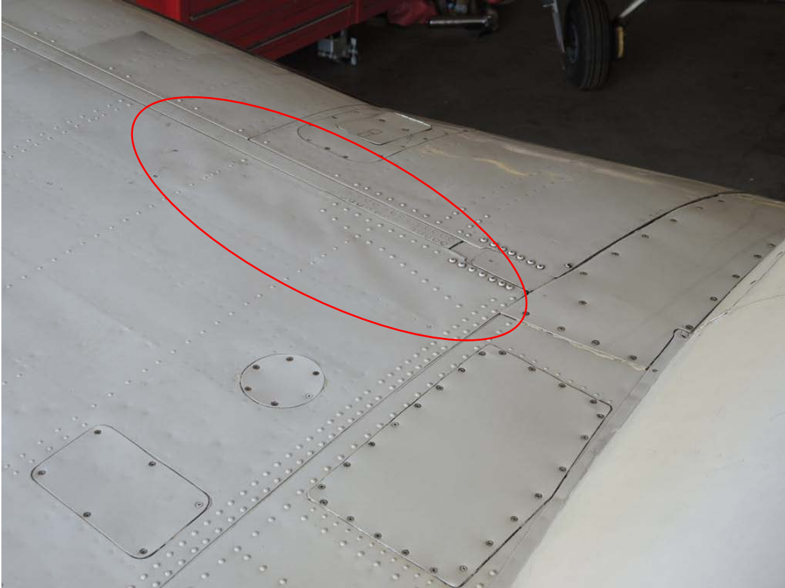
Figure 13. Close view of wrinkles in the top skin of the left wing, immediately outboard of the engine and aft of the forward spar, (Photo from: Textron Report ASI-16-CF, taken August 11, 2016)
