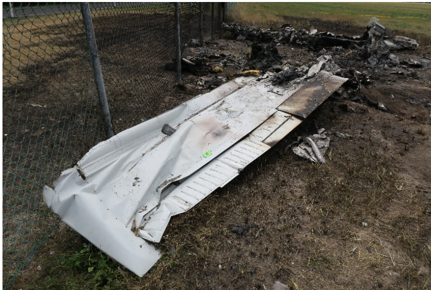
Figure 41. Right wing bottom surface prior to erecting tarps on the fence. Note the complete aileron, servo tab, and outboard flap. (Photo from: Textron)
