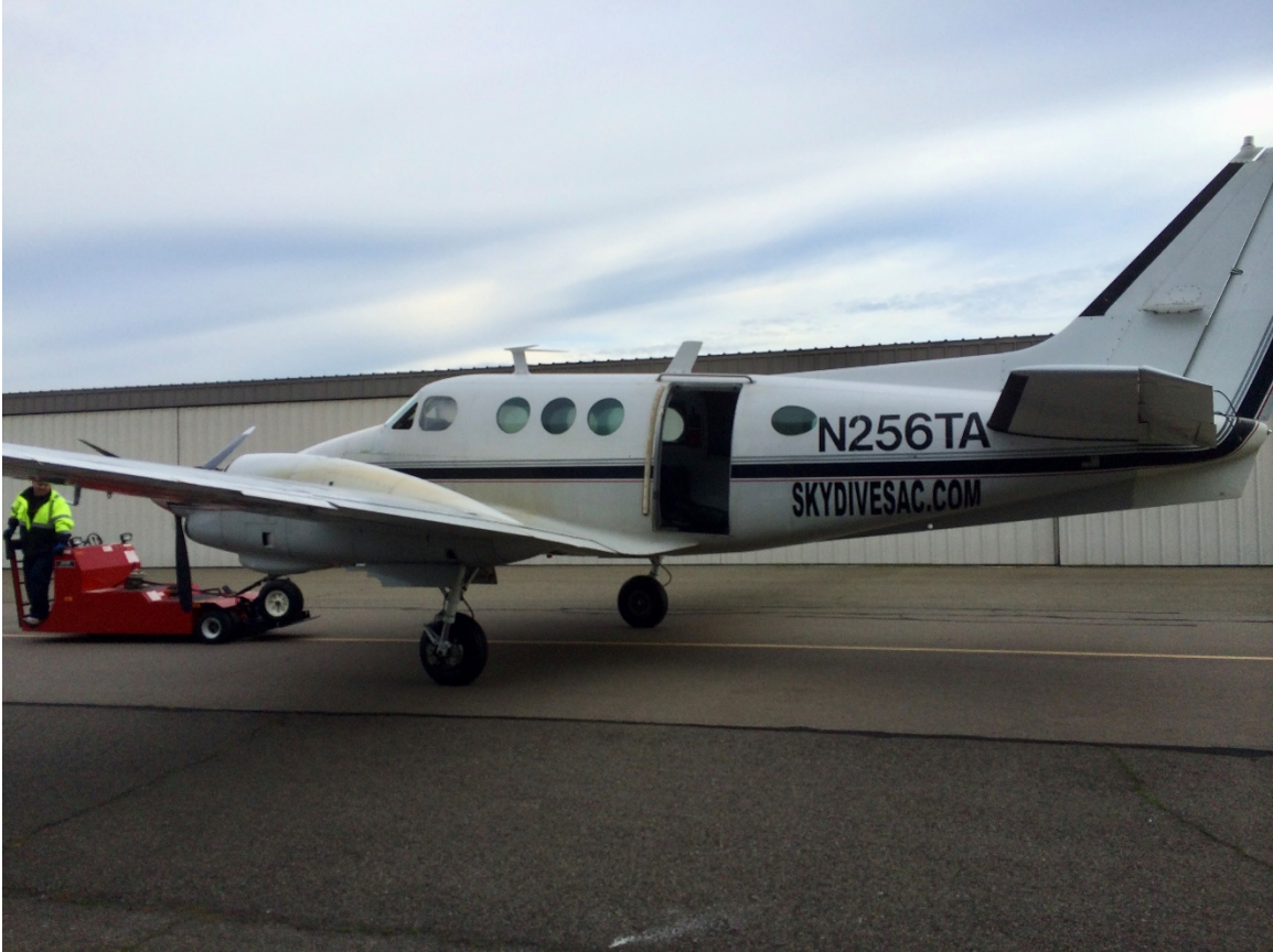
Figure 1 Accident aircraft being towed showing the aileron trim tab in a left wing down position
