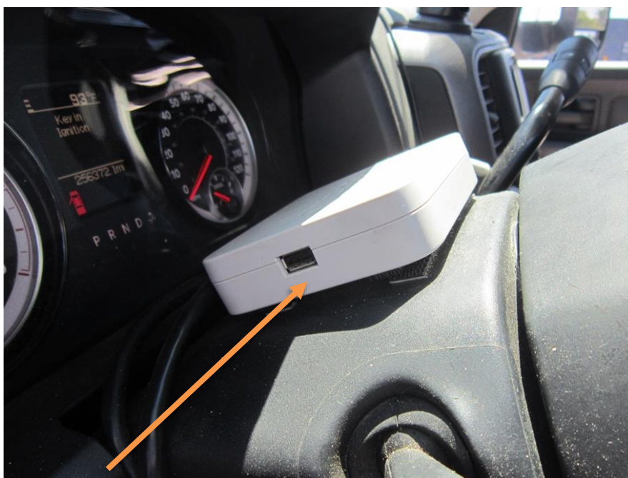
Photo 1. ABORD transmitter box. Orange arrow shows box disconnected.
