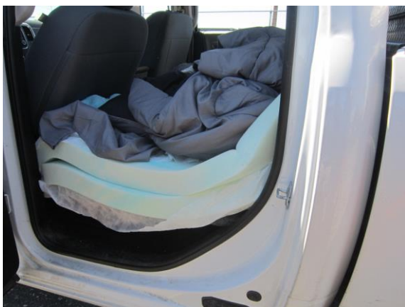
Images 2-3 Exemplar Vehicle with non-compliant sleeper berth. 19
