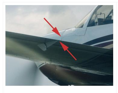
Detail: 2nd flap hinge on seam
