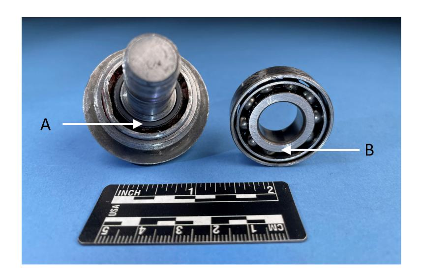
This picture is of the moisture seal removed from the eye bolt (left) and the upper bearing (right). Arrow A points to the elastomer seal of the moisture seal. Arrow B points to the inner race of the upper bearing.
