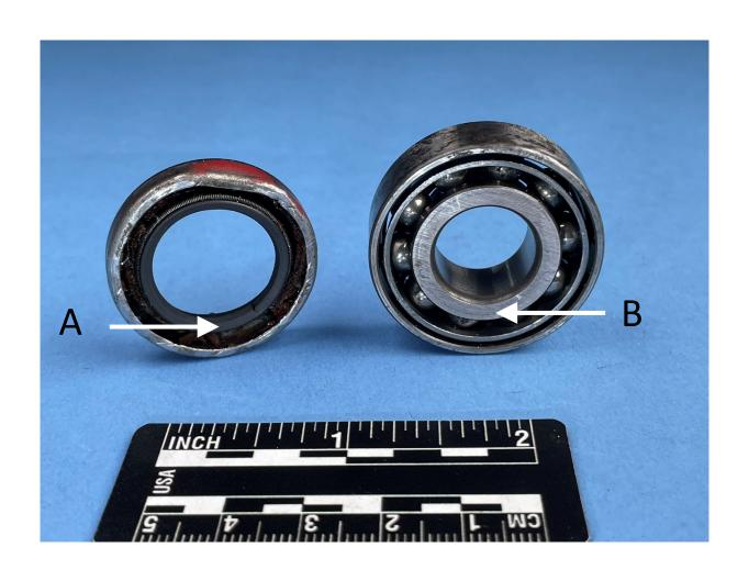
Two views showing how the moisture seal and upper bearing contacted each other. Note the moisture seal is resting on the inner race of the upper bearing, and the moisture seal sits just inside of the outer race of the upper bearing.
